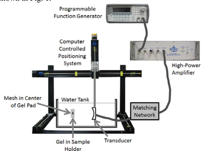
Fig. 1. Experimental setup illustrating the position of the mesh inside of the gel pad during the ultrasound exposures.
