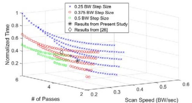
Fig. 11. Estimate of normalized time as a function of scan speed and the number of passes for three different step sizes.
