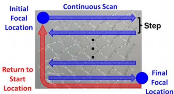
Fig. 4. Illustration of ultrasound exposure parameters where the focal spot was continuously scanned in the horizontal direction, stepped in the vertical direction, and passed over the mesh multiple times when treating the biofilms.
