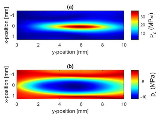
Fig. 3. (a) Peak compression,  $p_c$ , and (b) rarefactional,  $p_r$ , pressures in the focal region from the measurement/modelling calibration of the transducer.
