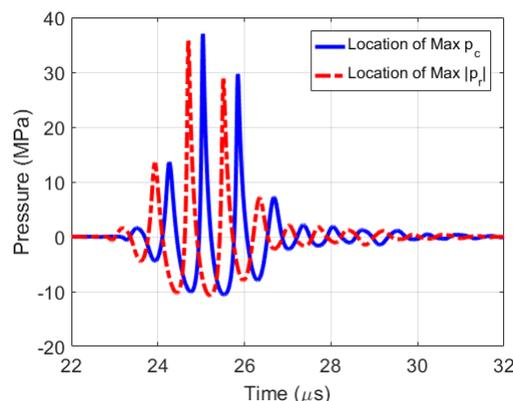
Fig. 2. Waveforms at the location of peak compressional pressure,  $p_c$ , and peak rarefactional pressure,  $p_r$ , found from the measurement/modelling calibration of the transducer.
