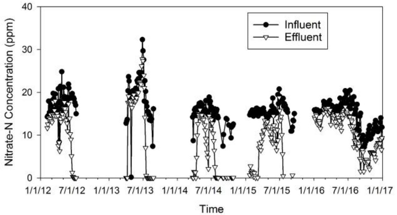
Figure 1. Nitrate-N concentrations in the bioreactor influent and effluent.
