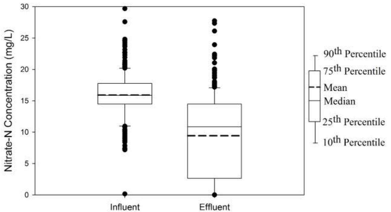
Figure 1. Box plot of nitrate-N concentrations in the influent and effluent from the bioreactor for 2012-2016.
