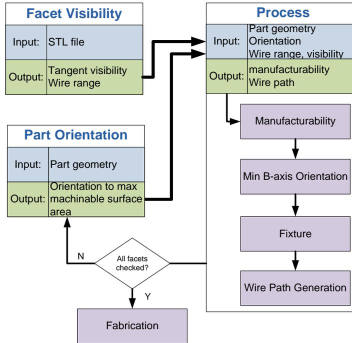
4. *Fabrication:* After analysis of all the facets in the STL file, the wire path will be sent to a 6-axis WEDM machine for fabrication the prototyping model.
