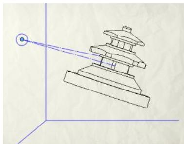
(a) Conventional visibility. Visibility from a point, such as visibility for milling process
