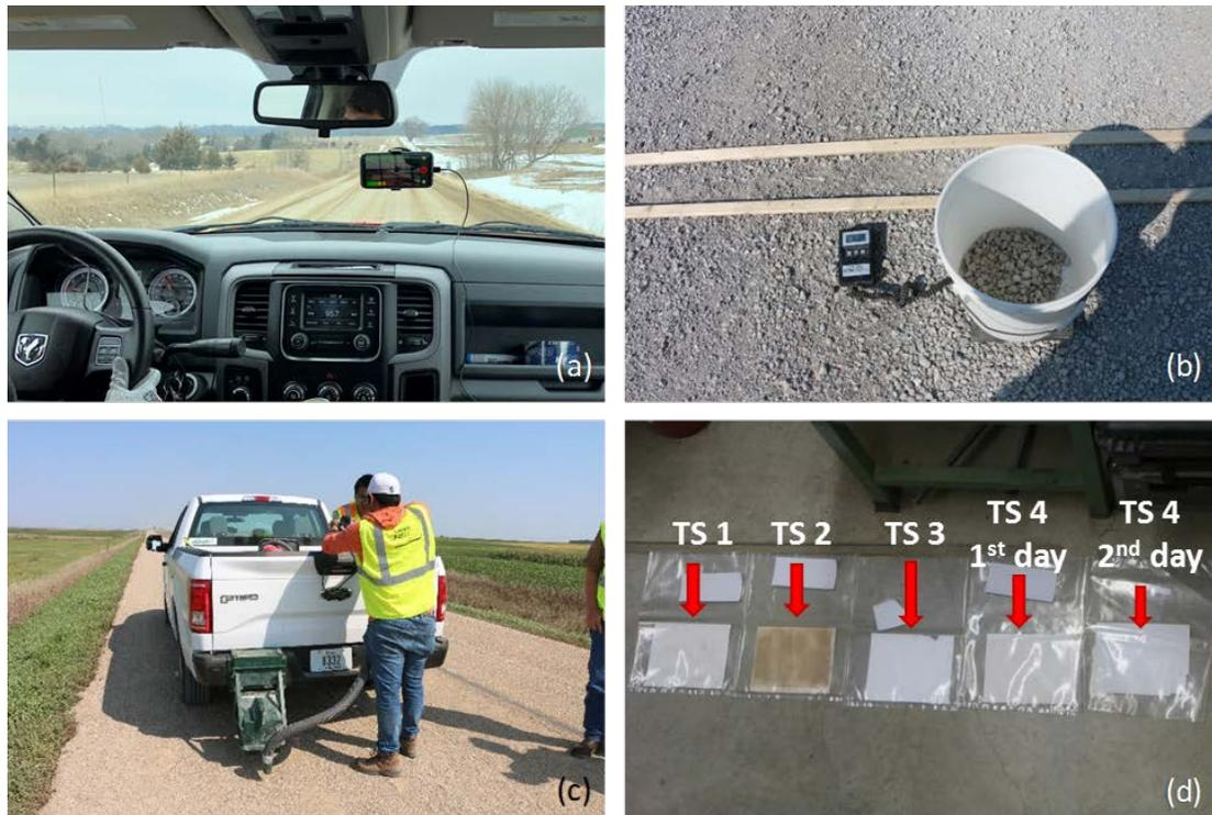
**FIGURE 4 (a) Measuring IRI using Roadroid software installed in a mobile phone, (b) loose aggregate test equipment, (c) installing dustometer test equipment, (d) filter papers from dustometer tests.**
