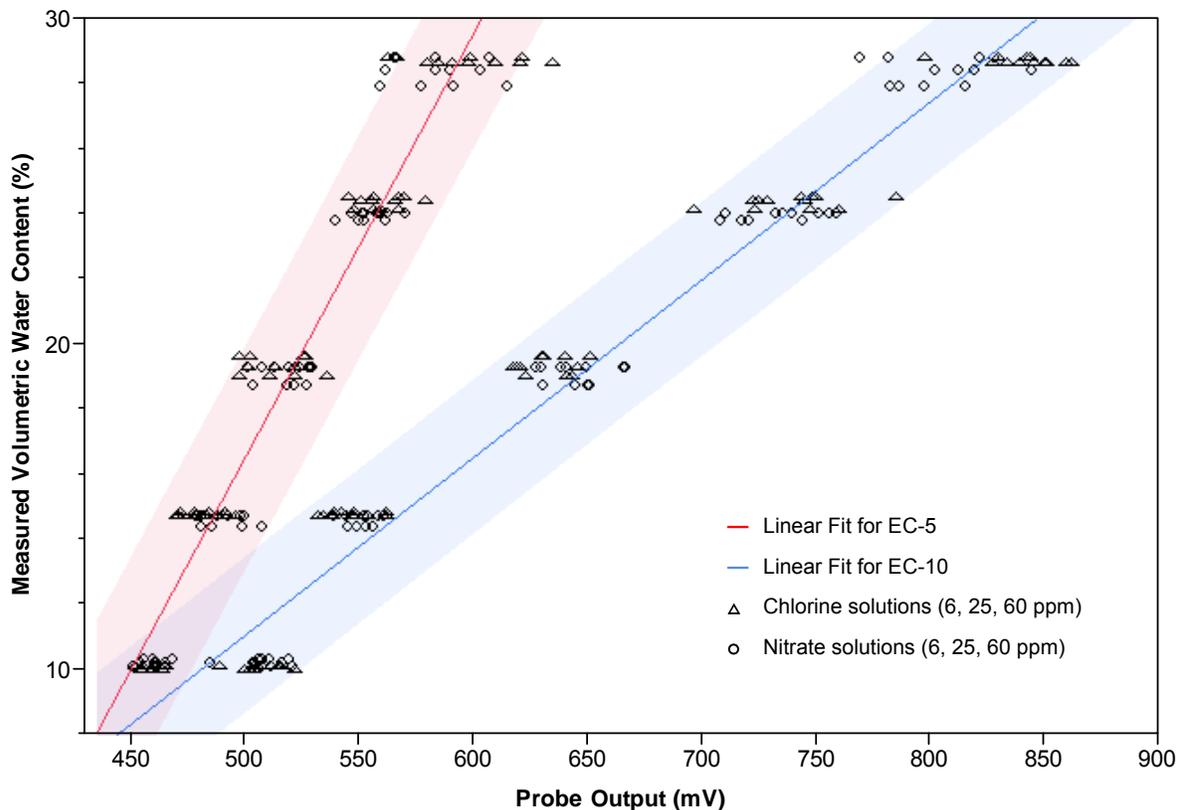
Figure 1. Relationship between VWC and the raw voltage output of EC-5 and EC-10 probes. The shaded areas represent 95% prediction intervals for each regression model.
