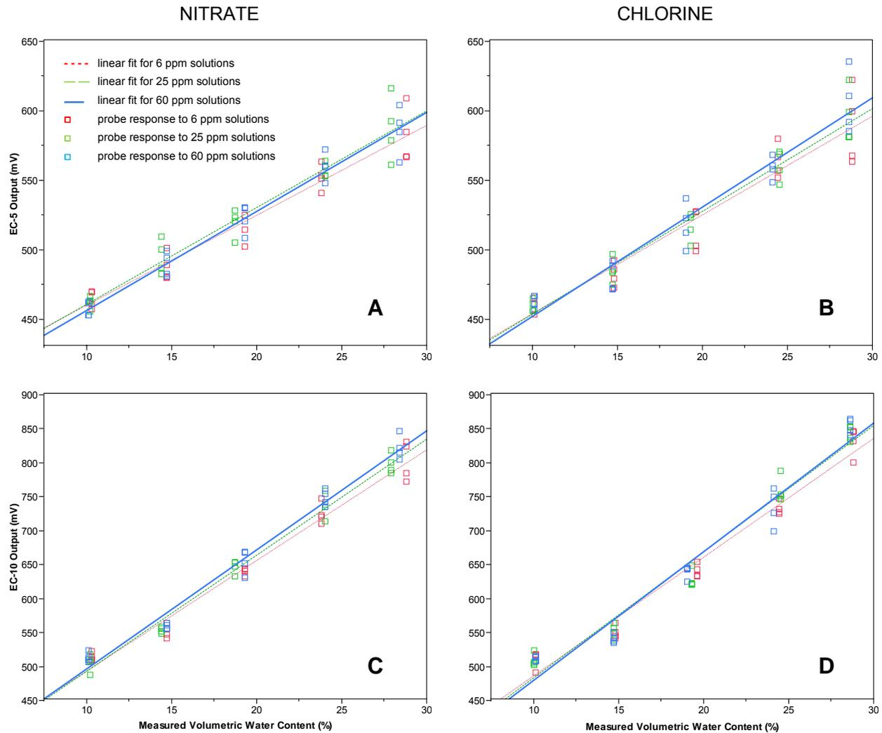
Figure 2. Response of the sensors to different concentrations of nitrate and chloride solutions: (A) and (B) response of EC-5 probes to nitrate and chloride solutions respectively, (C) and (D) response of EC-10 probes to nitrate and chloride solutions respectively
