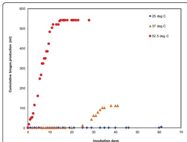
**Figure 4 Impacts of temperatures on biogas production.** The red solid circle indicates cumulative biogas production at 52.5°C, yellow triangles indicate biogas production at 37°C, and dark blue diamonds indicate biogas production at 25°C.
