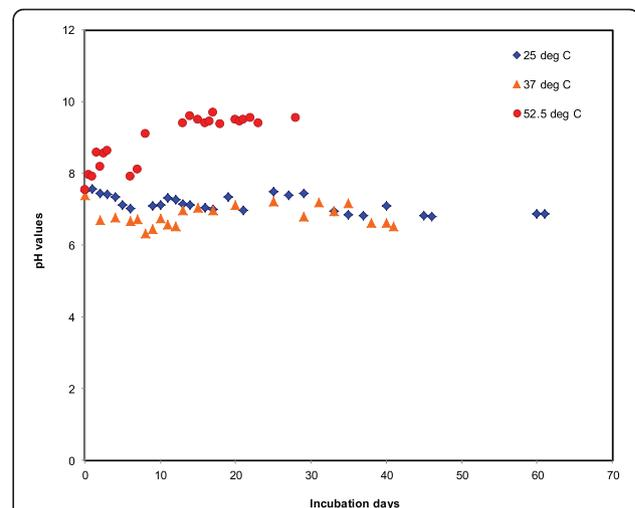
**Figure 5 Impacts of temperatures on pH changes.** The red solid red circle indicates pH changes at 52.5°C, yellow triangles indicate pH changes at 37°C, and dark blue diamonds indicate pH changes at 25°C.
