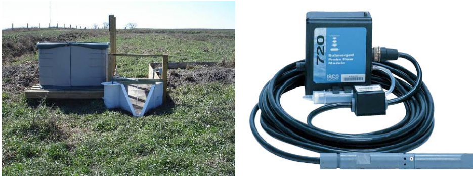
Figure 10. 0.46m outlet flume from a VTA (left) and the 720 submerged probe and module.
