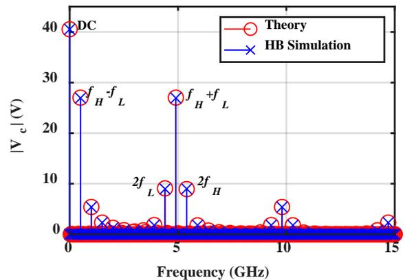
Fig. 3. Magnitude of complex Fourier series coefficients of the balun common-mode voltage, showing large IM2 components, derived analytically (red), and using Harmonic Balance simulation (blue), for  $I_{DC} \approx 2.5$  A,  $R_L = 100 \Omega$ ,  $f_L = 2.2$  GHz,  $f_H = 2.7$  GHz. The overlap between the two plots demonstrates the agreement between theory and simulation.
