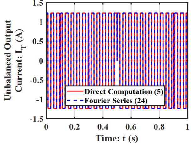
Fig. 2. Plot of unbalanced output current  $I_T(t)$  for one time period  $T_c = 1/f_c$  showing the equivalence of equations (5) and (24), assuming  $I_{DC} \approx 2.5$  A,  $R_L = 100$   $\Omega$ ,  $f_H/f_L = 27/22$ . In (24),  $k$  is restricted from 1 to 10000.
