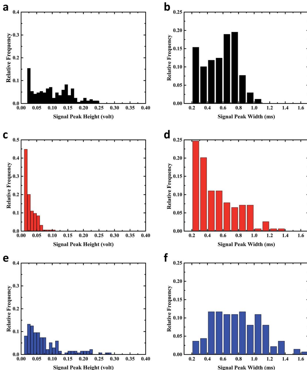
Fig. 4 (a and b) Signal peak heights and signal peak widths frequency distribution of 3.2  $\mu\text{m}$  microbeads. (c and d) Signal peak heights and signal peak widths frequency distribution of *Chlorella vulgaris*. (e and f) Signal peak heights and signal peak widths frequency distribution of *Chlorella protothecoides*. The signal peak height and the signal widths distribution of 3.2  $\mu\text{m}$  particles, *Chlorella vulgaris* and *Chlorella protothecoides* are different.
