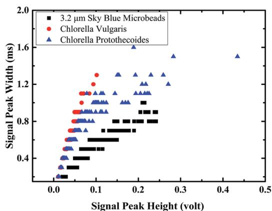
Fig. 5 Signal peak widths to signal peak heights of  $3.2 \mu\text{m}$  microbeads the *Chlorella vulgaris* and the *Chlorella protothecoides*. Data cluster of  $3.2 \mu\text{m}$  microbeads is distributed at different region as *Chlorella vulgaris* and the *Chlorella protothecoides*.
