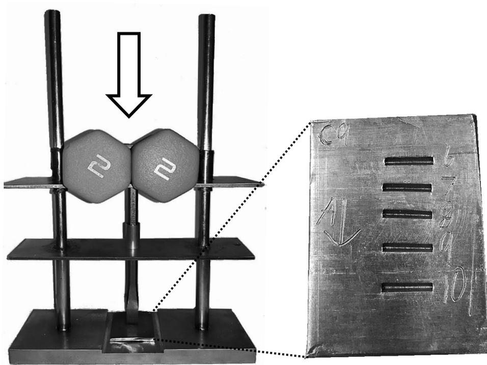
**Figure 2: Example of the jig, the direction of applied force and example impression marks.**
