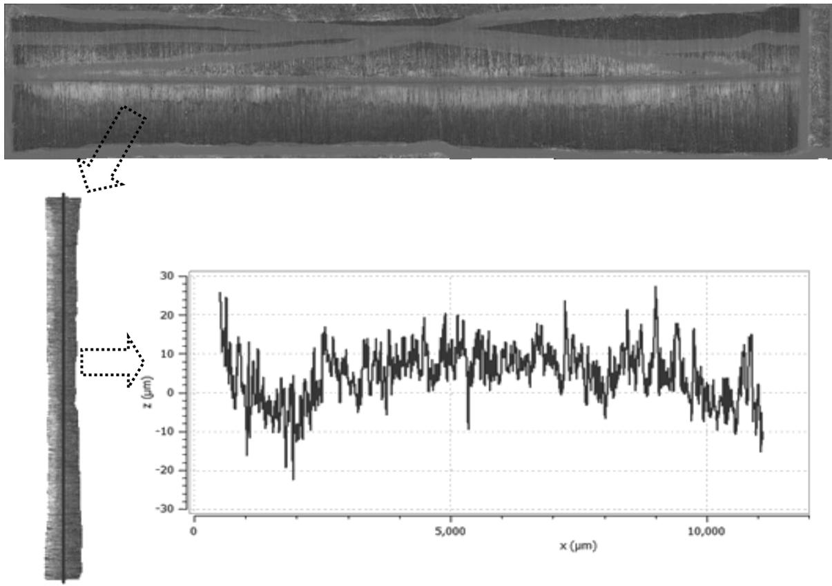
**Figure 4: Masking process and extraction of planar toolmark.**
