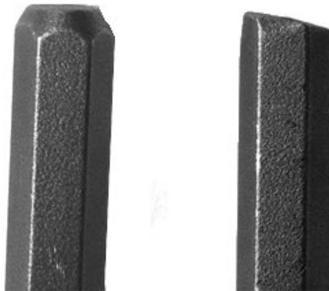
**Figure 8: Example of one chisel with a level striking end and one with an unlevel striking end.**
