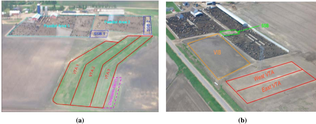
Figure 1. Diagrams of VTS configurations (a) solid settling basin – vegetative treatment area system (b) solid settling basin – vegetative infiltration basin – vegetative treatment area system
