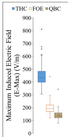
Fig. 7. Comparison of the maximum induced electric field, E-Max (V/m) on the head model between the FOE coil, QBC and THC.
