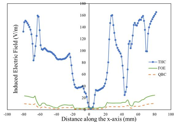
Fig. 6. Comparison of induced electric field along the x-axis on the transverse plane of the three coils.
