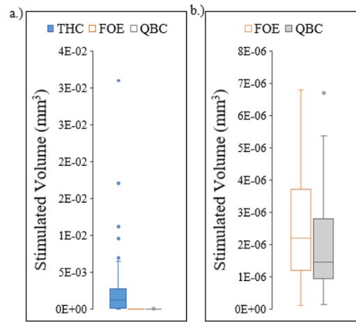
Fig. 8. Comparison of the stimulated volume, V-Half (mm<sup>3</sup>) on the head model between the (a) FOE coil, QBC and THC (b) FOE coil and QBC. Fig. 8b has been represented to give a better understanding of the comparison of the V-Half between the FOE coil and the QBC.
