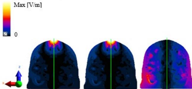
Fig. 3. Slice view along the z-axis of the Coronal Plane showing the induced electric field in the gray matter with the FOE coil (left), QBC (middle) and THC (right) on the head model. The surface plots have been normalized with the maximum value of the induced electric field that the FOE coil induces in the brain.
