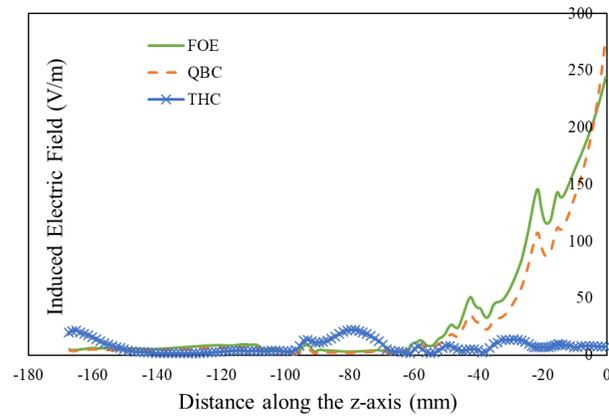
Fig. 4. Comparison of induced electric field along the z-axis on the coronal plane of the three coils.
