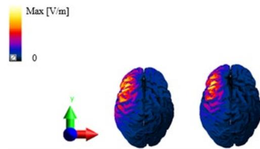
Fig. 9. Induced electric Field in the gray matter by the FOE coil (left) and QBC (right) at the left DLPFC location of the head model. The surface plots have been normalized with the maximum value of the induced electric field that the FOE coil induces in the brain.
