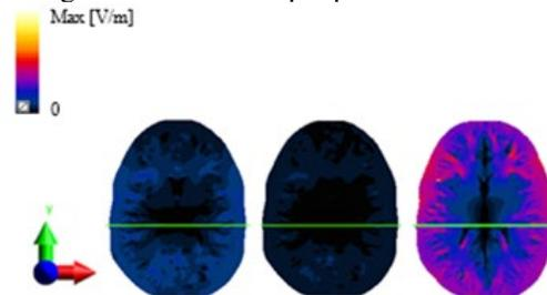
Fig. 5. Slice view along the x-axis of the Transverse Plane showing the induced electric field in the gray matter with the FOE coil (left), QBC (middle) and THC (right) on the head model. The surface plots have been normalized with the maximum value of the induced electric field that the FOE coil induces in the brain.
