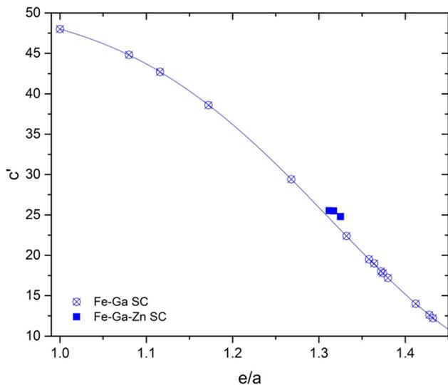
FIG. 2. Shear modulus,  $c'$ , vs. electron to atom ratio,  $e/a$ , for Fe-Ga and Fe-Ga-Zn. Lowering the  $e/a$  by ternary additions of Zn to Fe-Ga slightly increases  $c'$ . The line is included as a guide to the eye. Binary data are from Ref. 2.
