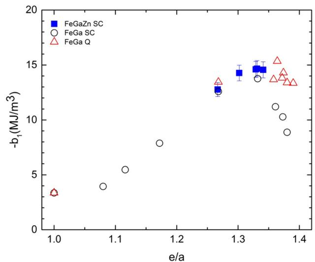
FIG. 3. Magnetoelastic coupling coefficient,  $-b_1$ , vs. electron-to-atom ratio,  $e/a$ , for SC and quenched (Q), (100) single crystal samples. Lowering the  $e/a$  by ternary additions of Zn to Fe-Ga slightly improves  $-b_1$ . Binary data are from Ref. 2.
