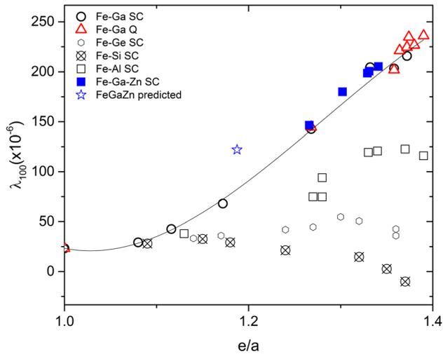
FIG. 1. Magnetostriction,  $\lambda_{100}$ , vs. electron to atom ratio,  $e/a$ , for Fe-X alloys. The line is included as a guide to the eye. All binary data are from Ref. 2. Predicted data point is from Ref. 6.
