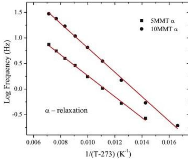
Fig. 10: The linear dependence of  $\log f$  of  $\alpha$ -relaxation of 5MMT and 10MMT on  $1/(T-273)$ .
