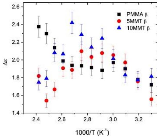
Fig. 11:  $\Delta\epsilon$  of the  $\beta$ -relaxation of PMMA, 5MMT, and 10MMT as a function of reciprocal temperature.
