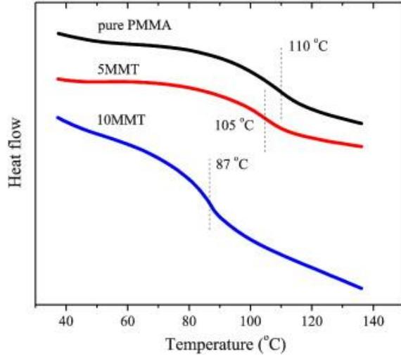
Fig. 9: DSC thermogram of PMMA and nanocomposites.
