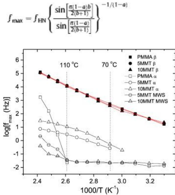
Fig. 8: Arrhenius diagram showing  $\alpha$  -,  $\beta$  -, and MWS relaxations of PMMA, 5MMT, and 10MMT.
