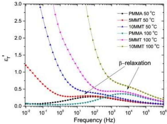
Fig. 5: The imaginary relative permittivity of PMMA, 5MMT, and 10MMT as a function of frequency at 50 and 100 °C.
