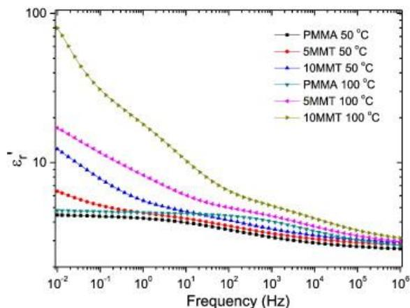
Fig. 4: The real relative permittivity of PMMA, 5MMT and 10MMT as a function of frequency at 50 and 100 °C. For clarity, only these two (out of thirteen) measured temperatures in the range from 30 to 140 °C, at 10 °C increments, are plotted here.
