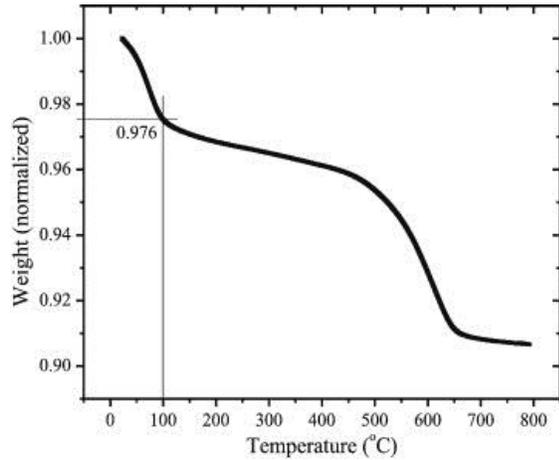
Fig. 1: Normalized weight of MMT while heated from 20 to 800 °C at a heating rate of 20 °C/min.
