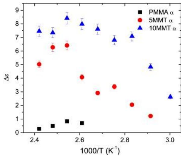
Fig. 12:  $\Delta\epsilon$  of the  $\alpha$ -relaxation of PMMA, 5MMT, and 10MMT as a function of reciprocal temperature.
