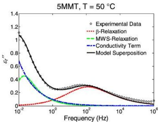
Fig. 6: Model fitting of the imaginary relative permittivity of 5MMT at 50 °C.
