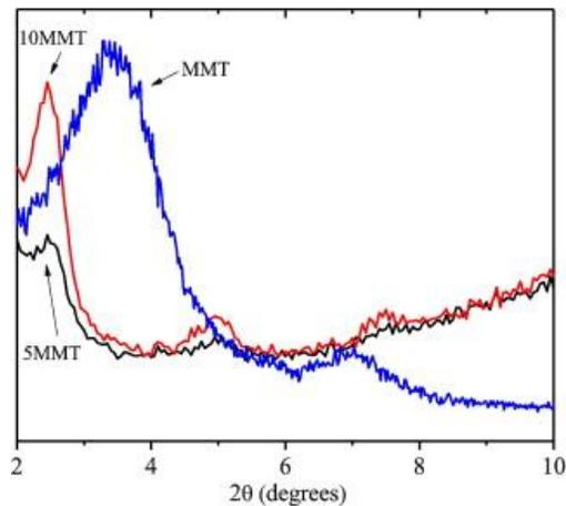
Fig. 3: XRD spectra of 5MMT, 10MMT and pure MMT.
