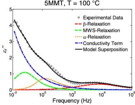
Fig. 7: Model fitting of the imaginary relative permittivity of 5MMT at 100 °C.
