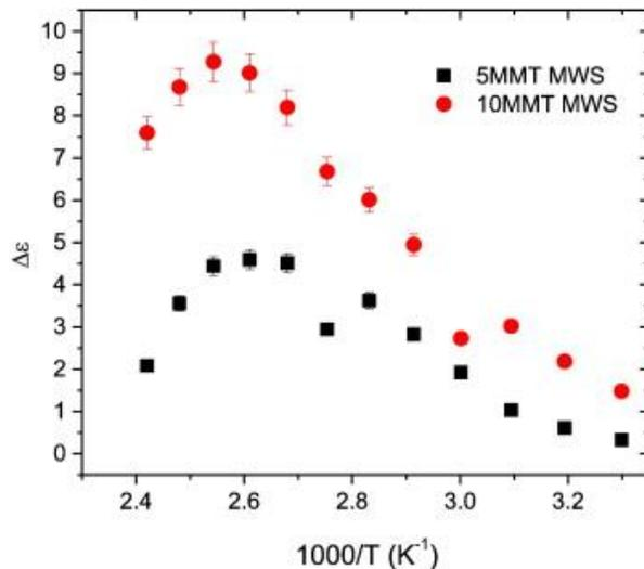
Fig. 13:  $\Delta\epsilon$  of the MWS relaxation of 5MMT and 10MMT as a function of reciprocal temperature.
