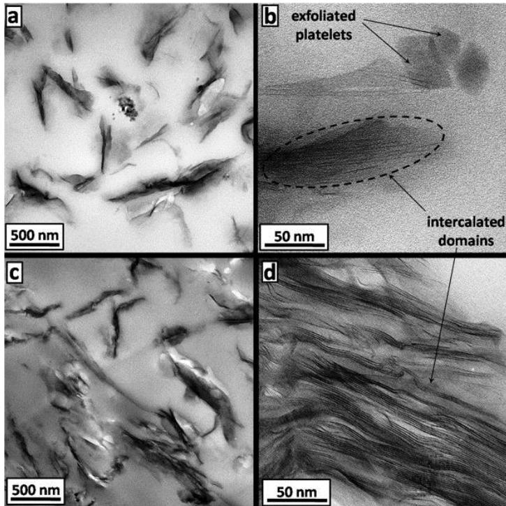
Fig. 2: TEM images of 5MMT (a and b) and 10MMT (c and d).
