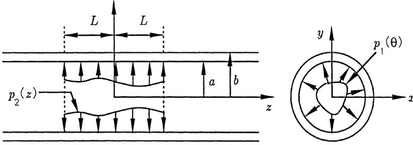
Fig. 1. Geometry of loaded cylinder.
