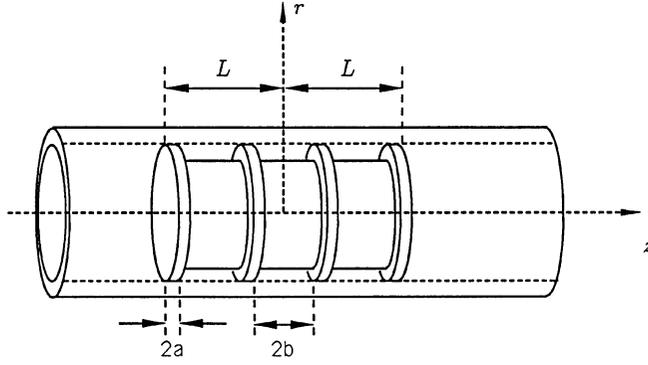
Fig. 3. Typical comb type transducer with  $N = 4$  "fingers".
