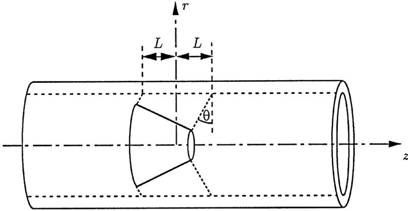
Fig. 2. Typical wedge type transducer
