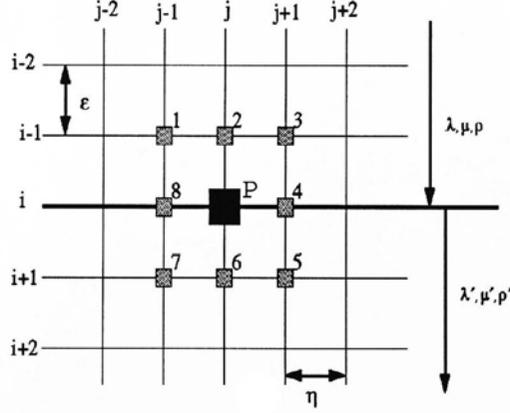
Fig. 1. Processors utilized for iteration equation at time  $t+1$  at the point P. The interface shown here, passes through point P, along  $i$ .
