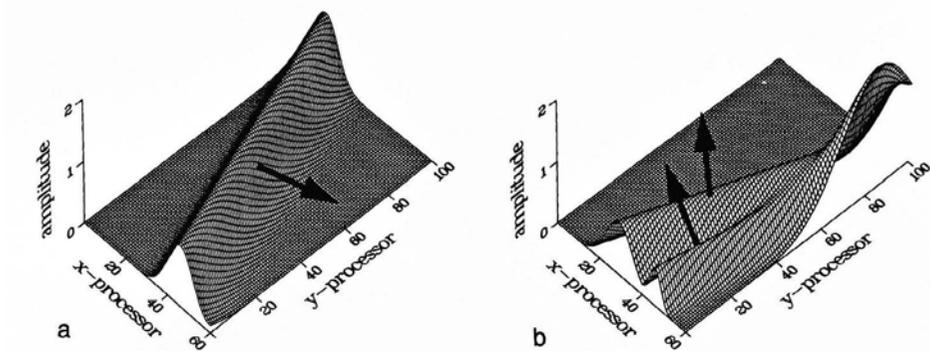
Fig. 2. A longitudinal wave, gaussian in time and infinite in extent, propagated at 20 degrees with respect to the normal of the free boundary. a) Shows the wave approaching the boundary, b) shows the reflected longitudinal and shear waves.
