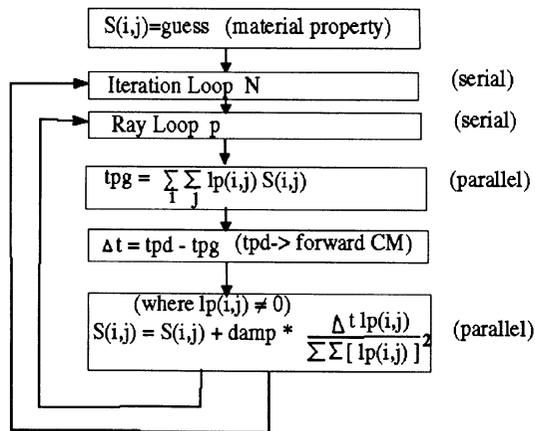
Fig. 5. Flow chart of the modified ART type routine being used. Areas that are parallel and those that are still serial are indicated.
