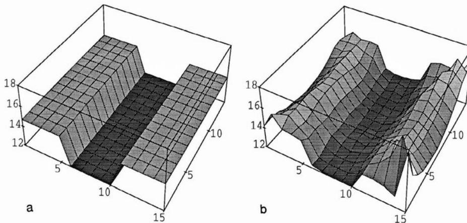
Fig. 4. a) Simulated, three-layer material. b) Reconstructed tomogram of the three-layer material. Vertical units are arbitrary.
