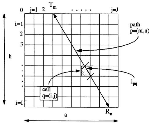
Fig. 3. Grid for reconstructing tomogram. Path  $p$  goes from  $T_m$  to  $R_n$ , passes through cell  $q=(i,j)$ . Distance of path  $p$  in cell  $q$  is  $l_{pq}$ .
