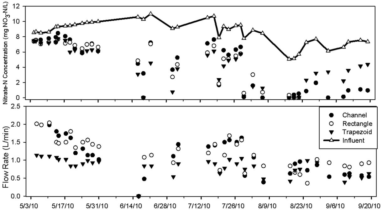
Figure 2. Influent and effluent NO<sub>3</sub><sup>-</sup>-N concentrations (a) and associated flow rates (b) for three pilot scale bioreactors filled with municipal yard waste operated during summer 2010.
