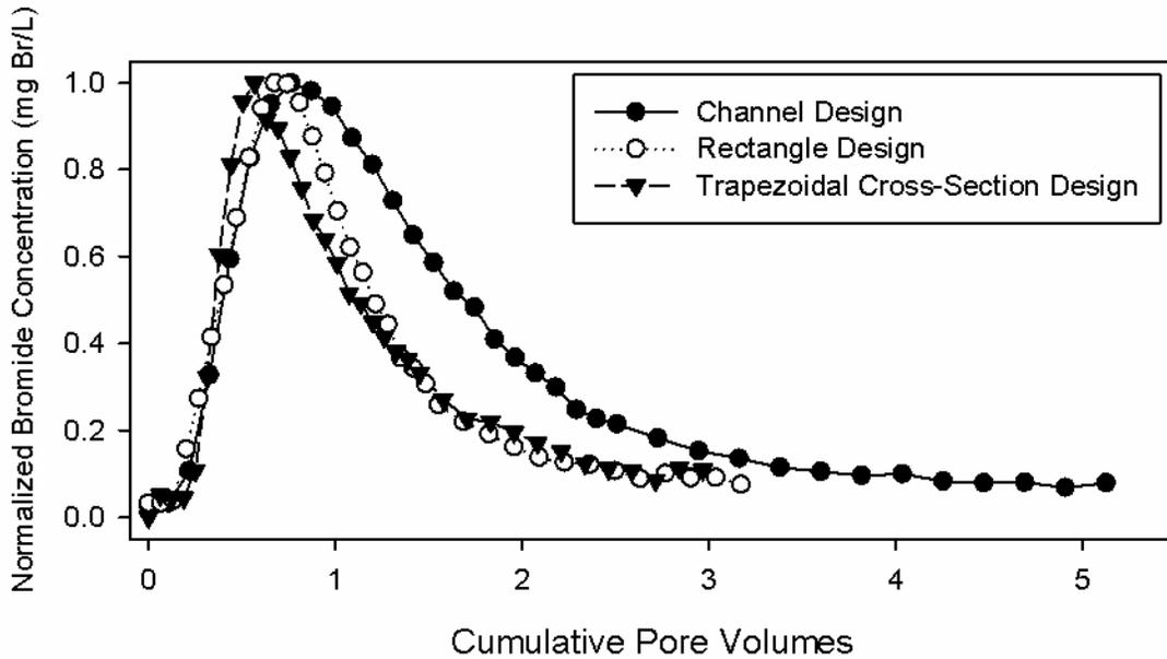
Figure 4. Normalized bromide tracer concentrations for three pilot bioreactors with yard waste as fill material.
