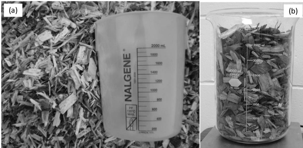
Figure 1. Yard waste used in pilot bioreactor study (a) and woodchips used in previous pilot bioreactor study (b). Note difference in beakers used for size reference: 2000mL beaker for yard waste (a) and 3500 mL beaker shown by “standard” woodchips (b).
