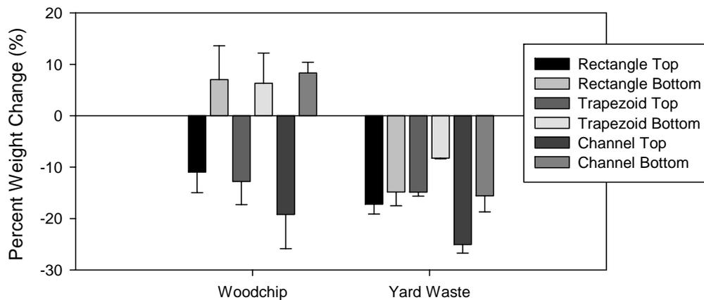
Figure 6. Weight change in buried media bags containing woodchips (Year 1) or yard waste (Year 2) after one summer of pilot bioreactor operation.
