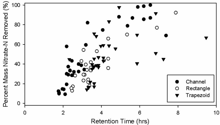
Figure 3. Retention time correlation with mass  $\text{NO}_3^-$ -N removal for three pilot-scale bioreactors.
