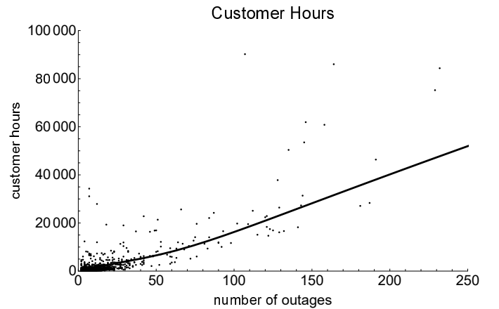
Fig. 11. Curve shows mean customer hours \bar{A} calculated from (28) versus number of outages. Dots show customer hours A of the events in the data.
