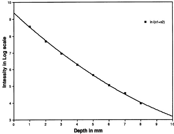
Figure 4. The natural logarithm of the transscatter intensity vs the steel thickness, obtained at a tube voltage of 160 KV for the case where  $x_1 = x_2$ .
