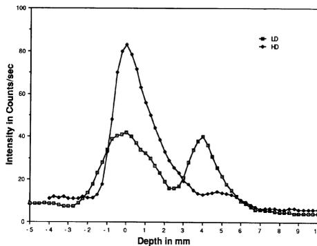
Figure 7. The density profile of high density (HD) and low density (LD) rust obtained at a tube voltage of 160 KV, 45° incident angle, 45° exit angle.
