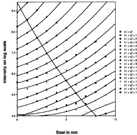
Figure 6. Family of curves of the intensity vs steel thickness for a constant sum  $x_S = x_1 + x_2$  as indicated in the legend. Also shown is the graph for  $x_j = x_S$ , from figure 5.
