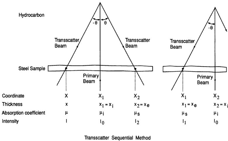
Figure 5. Definitions of the various parameters as used in the text. The right hand figure shows the situation after the incident beam has been shifted from  $X_1$  to  $X_2$ .
