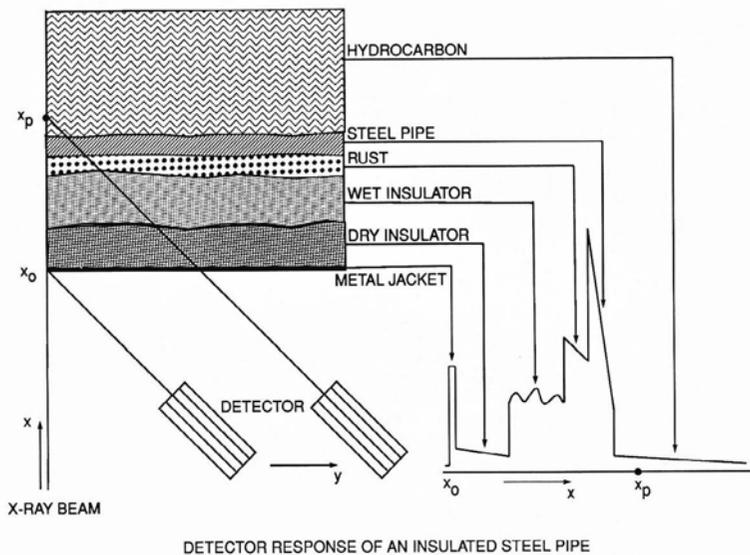
Figure 2. The geometrical arrangement of the x-ray source and the detector for the backscatter technique as described in the text. The ideal density profile of a typical insulated pipe is also shown.
