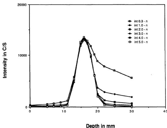
Figure 3. Experimental density profile for steel of various thickness, followed by paraffin, obtained at a tube voltage of 160 KV.
