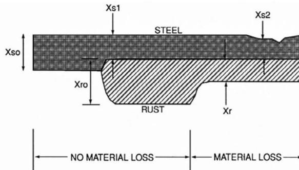
Figure 1. Steel losses due to corrosion and erosion;  $x_{s0}$  represents the thickness of the original steel wall,  $x_{r0}$  the thickness of the rust layer without loss of material,  $x_{s1}$  the wall thickness of the unaltered portion of the pipe,  $x_r$  the rust thickness when partial loss occurs, and  $x_{s2}$  the wall thickness of the pipe due to both erosion and corrosion.
