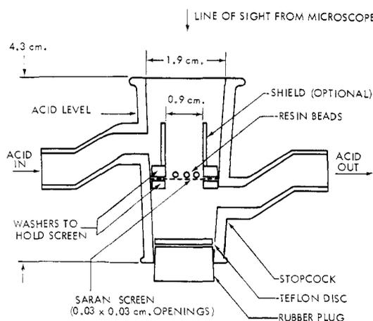
Figure 4. Cell used for eluting the resin beads
