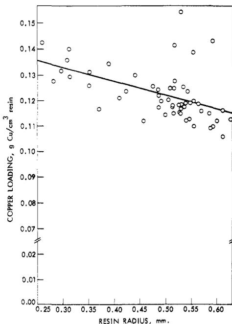
Figure 3. The copper content or loading of individual Dowex HCR-M resin beads
