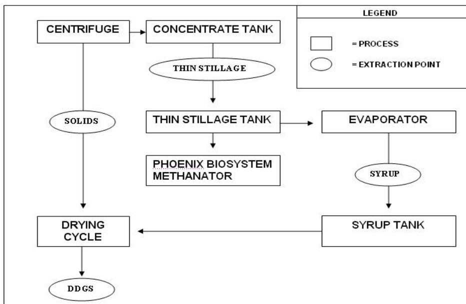
Figure 1. Diagram of co-products including DDGs, solids, syrup and thin stillage created after centrifuge step during corn to ethanol process.
