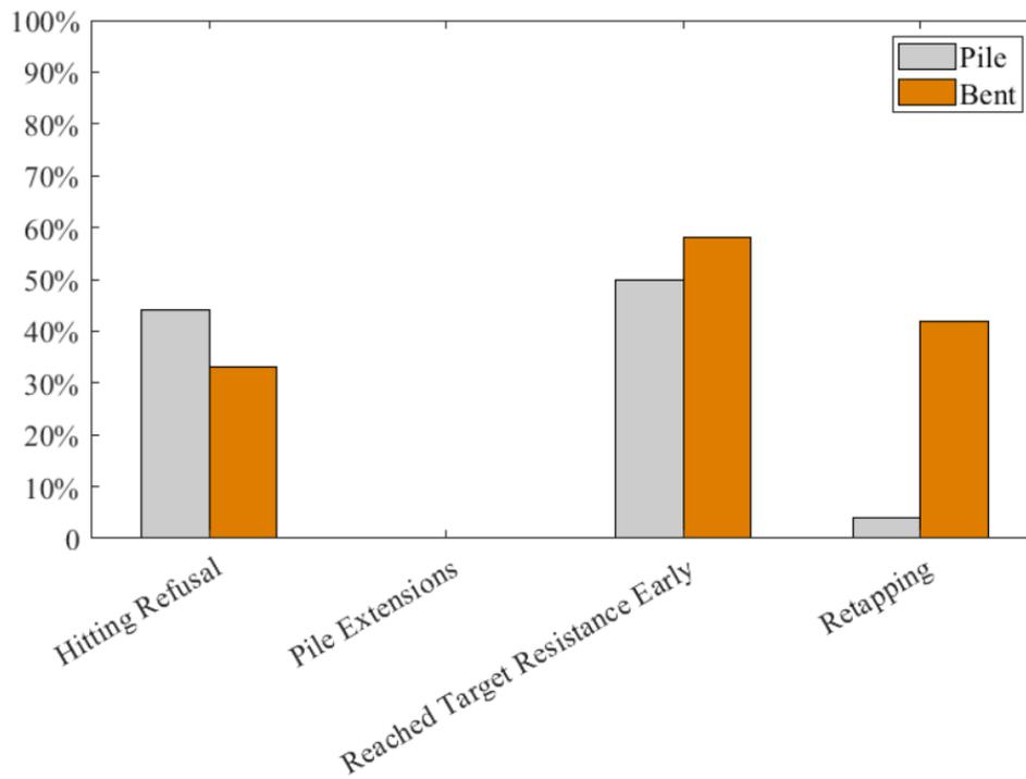
**Fig. 7.** Percentages of Variables Examined For Piling in Non-Cohesive Soils
