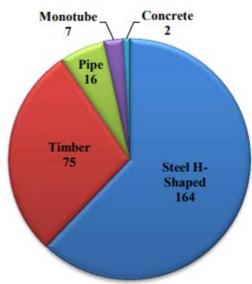
Fig. 1. Distribution of Iowa Past Pile Static Load Tests by Pile Type (Data from Roling et al. 2010)
