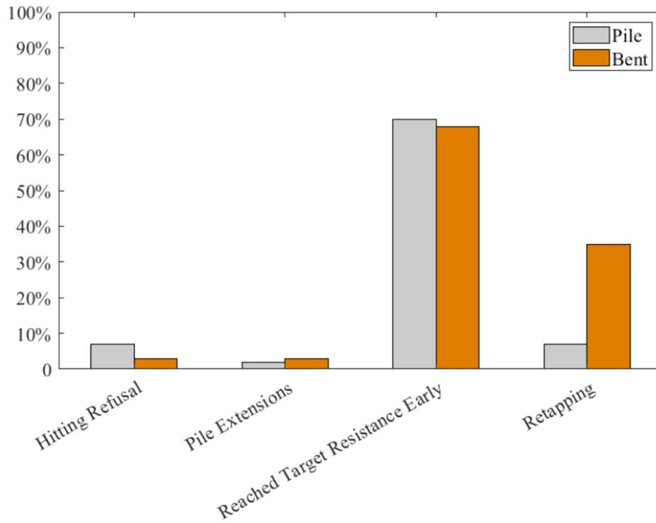
**Fig. 6.** Percentages of Variables Examined For Piling in Mixed Soils
