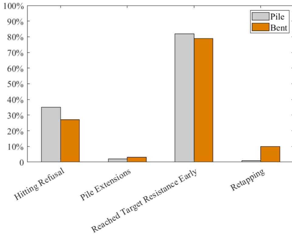
**Fig. 5.** Percentages of Variables Examined For Piling in Cohesive Soils
