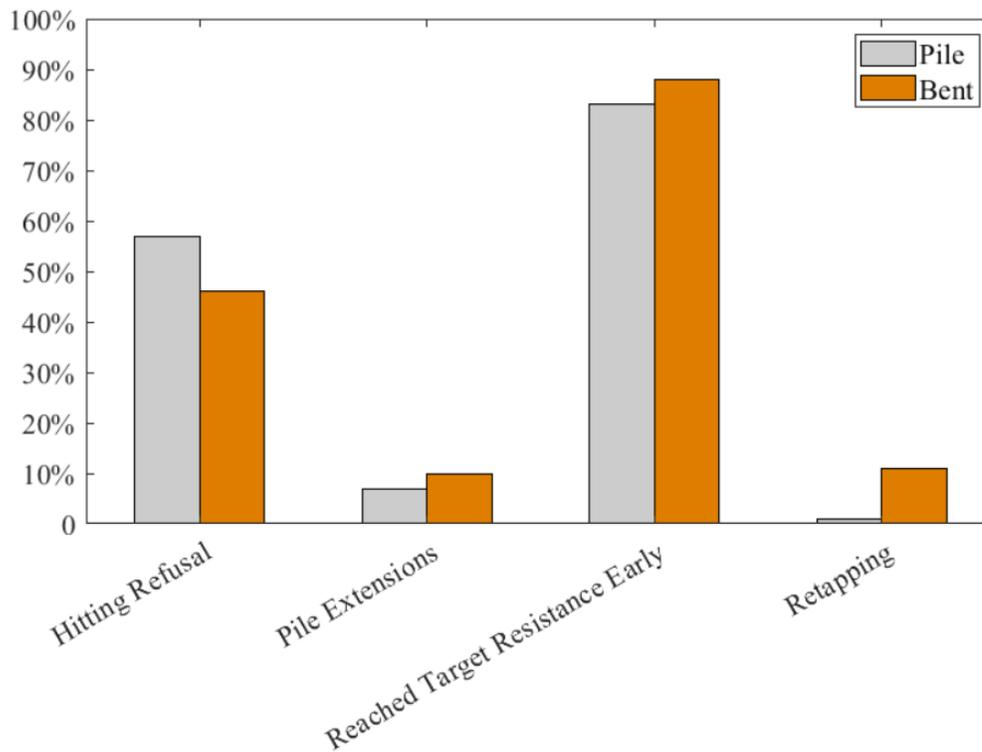
**Fig. 8.** Percentages of Variables Examined For Piling in Rock
