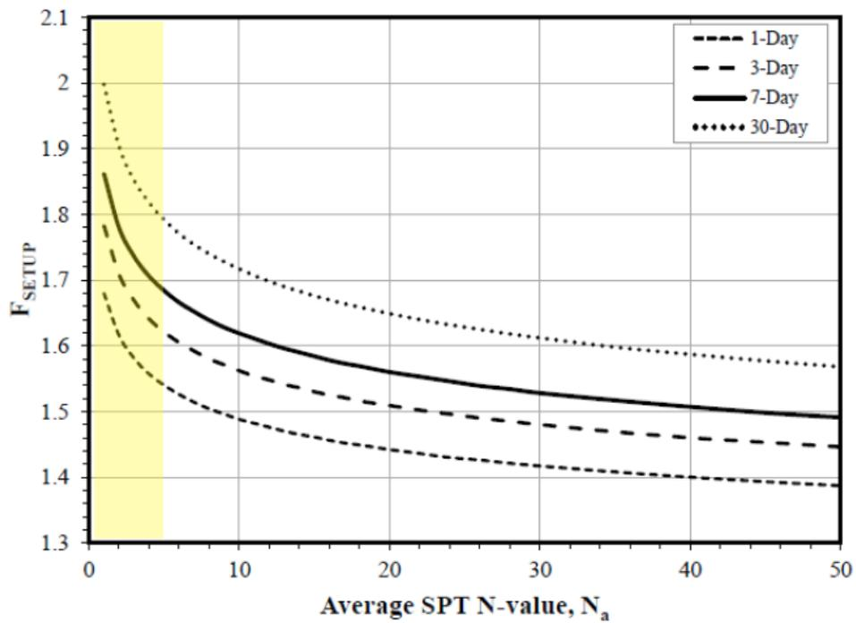
Fig. 3. Setup Factor Chart for Cohesive Soils (Data from Iowa DOT 2011)
