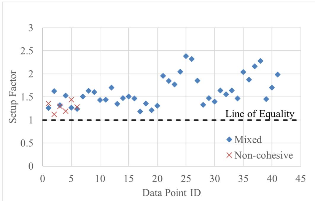
**Fig. 9.** Setup Factor in Mixed and Non-cohesive Soils
