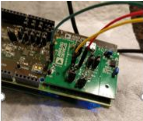
Figure 19: Wires from the pogo pin connected to the board
