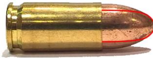
FIG. 5. A 9 mm Luger copper full metal jacket bullet and cartridge casing used in the experiment with the ovoid of Rankine shown by the line superimposed on its leading edge.
