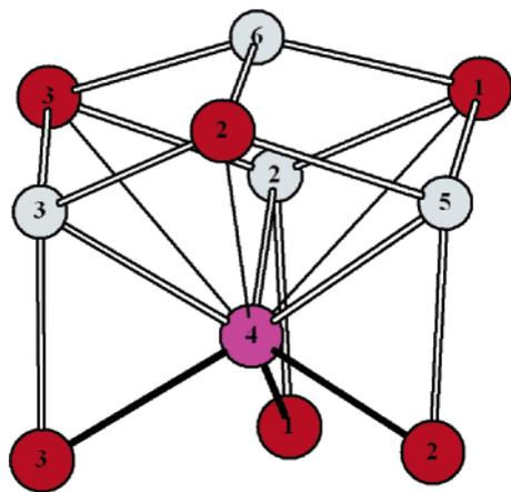
**Figure 7.** Geometric environment of the unique Sb4 (lavender), which is bonded within the ring to the lower Sb1, Sb2, and Sb3 atoms (3.22–3.25 Å) and distantly to the Sb1, Sb2, and Sb3 atoms in two other chains above (light lines) (at 4.20–4.28 Å) via intervening Na2, Na3, and Na5 atoms ( $d(\text{Sb}-\text{Na}) = 3.20\text{--}3.25$  Å). The Na6 cap is 3.83 Å from Sb4. The upper Na and Sb atoms appear to give good definition of a cavity presumably occupied by a lone pair of electrons on Sb4.
