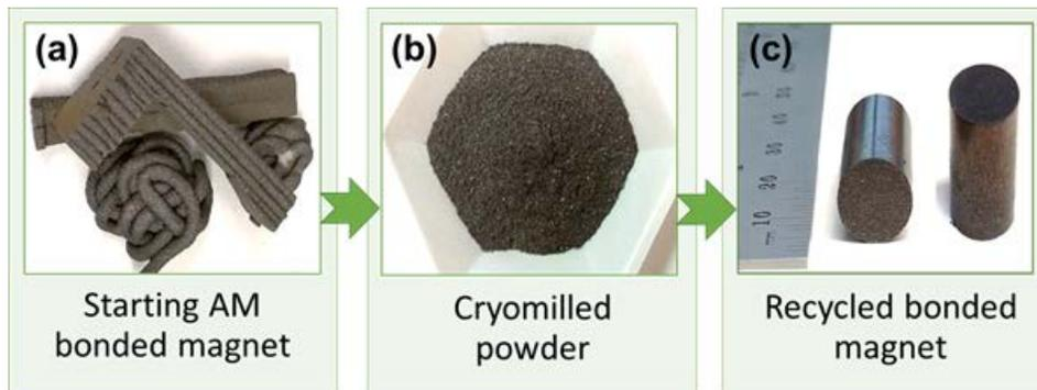
**Fig. 1.** (a) Starting AM bonded magnets (65 vol.% Nd-Fe-B in nylon), (b) cryomilled powder, and (c) recycled bonded magnets.
