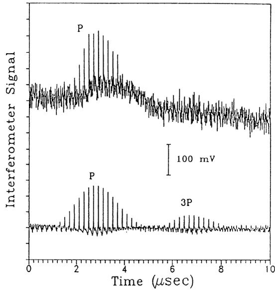
Fig. 3. Effect of narrowband (Weiner) filtering of a laser-generated ultrasonic signal produced by multiple pulsing at a single point.
