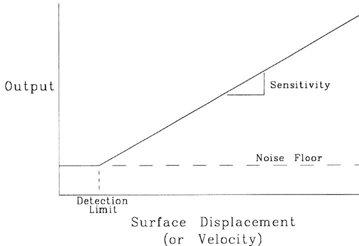
Fig. 1. Generalized transducer response curve.
