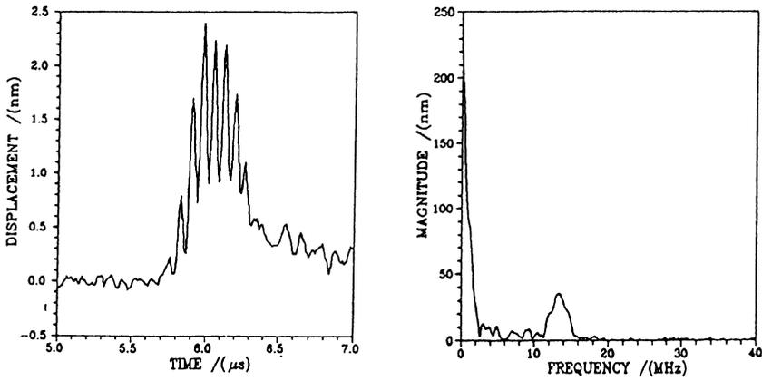
Fig. 2. Narrowbanding of acoustic signals using an array of laser line sources.
