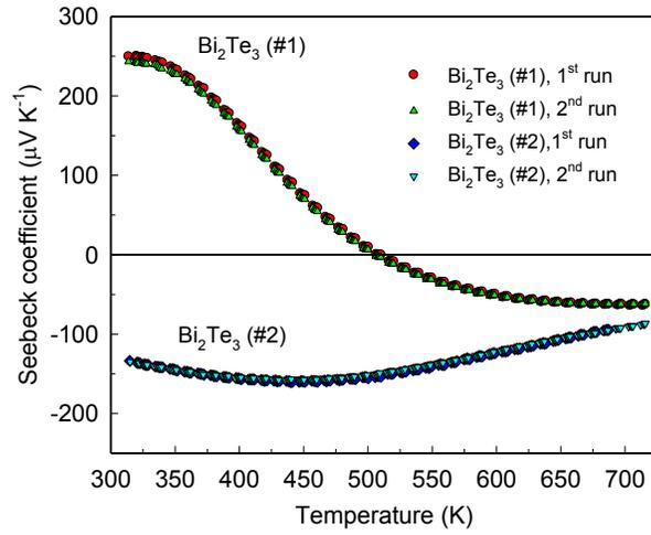
Figure 2. Temperature dependencies of the absolute Seebeck coefficient of Bi<sub>2</sub>Te<sub>3</sub> samples #1 and #2, showing stability of the Seebeck coefficient and different type of conductivity at 300 K.
