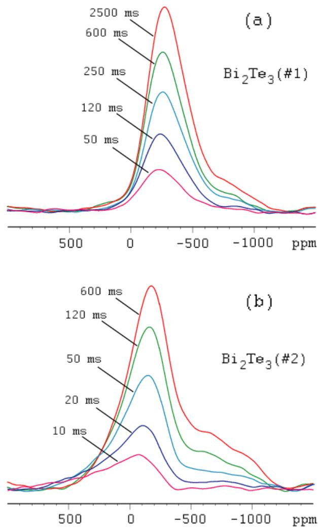
Figure 3.  $^{125}\text{Te}$  NMR spectra of  $\text{Bi}_2\text{Te}_3$  samples (a) #1 and (b) #2 obtained at 300 K for various saturation recovery (delay) times.
