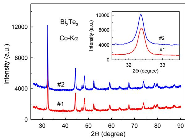
Figure 1. XRD ( $\text{Co-K}\alpha$ ,  $\lambda = 0.1789$  nm) patterns of  $\text{Bi}_2\text{Te}_3$  samples #1 and #2 at 300 K. The inset shows an expanded view for the main peak at  $31.5^\circ \leq 2\theta \leq 33.5^\circ$ .
