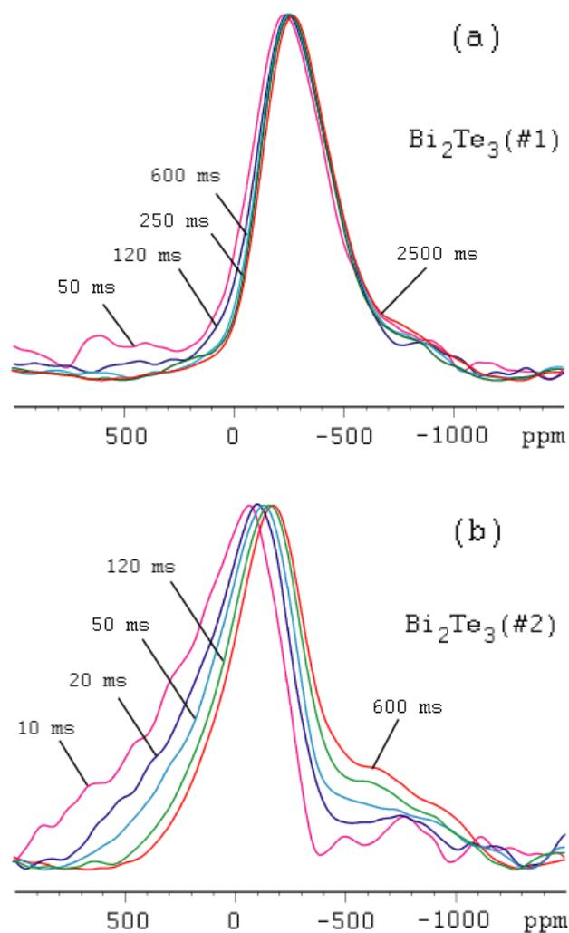
Figure 4.  $^{125}\text{Te}$  NMR spectra of  $\text{Bi}_2\text{Te}_3$  samples (a) #1 and (b) #2 obtained at 300 K for various saturation recovery (delay) times and rescaled to the value obtained for the saturated spectra.
