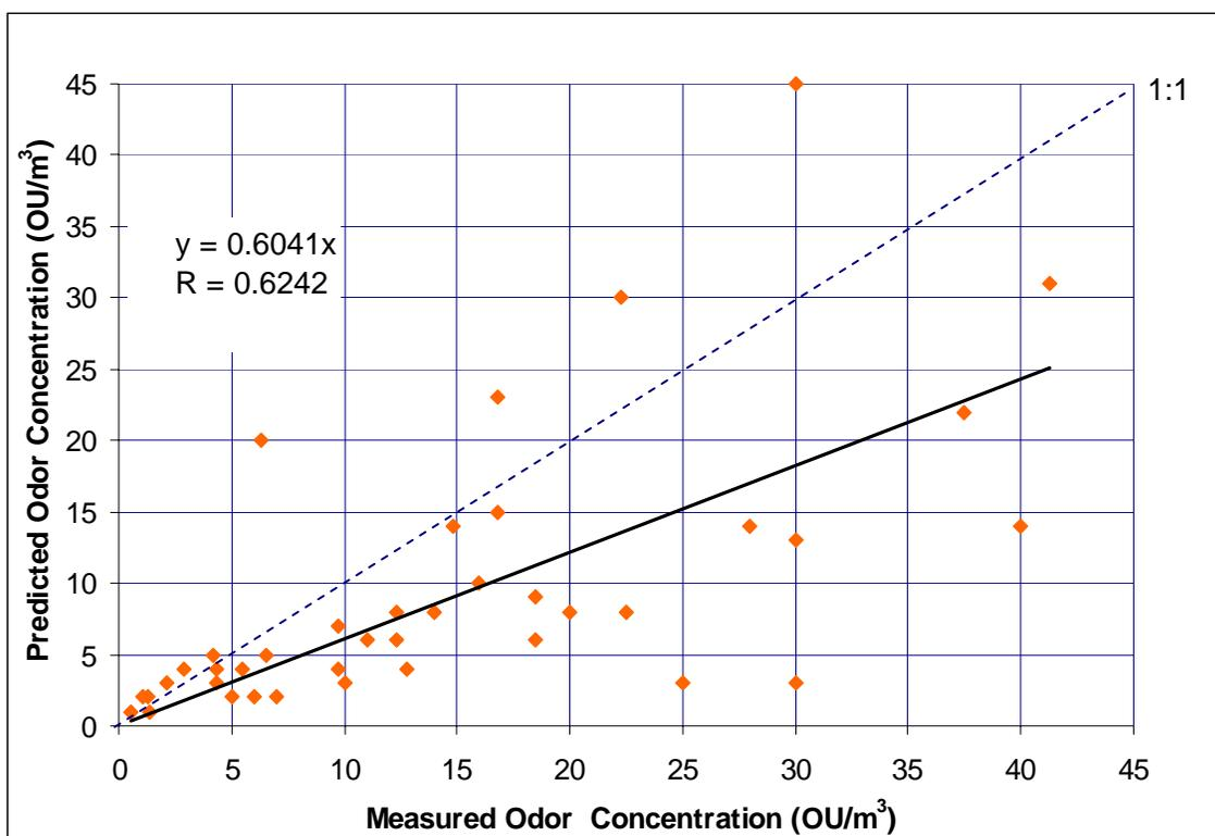
**Figure 2. Point source predicted versus measured odor concentrations.**
