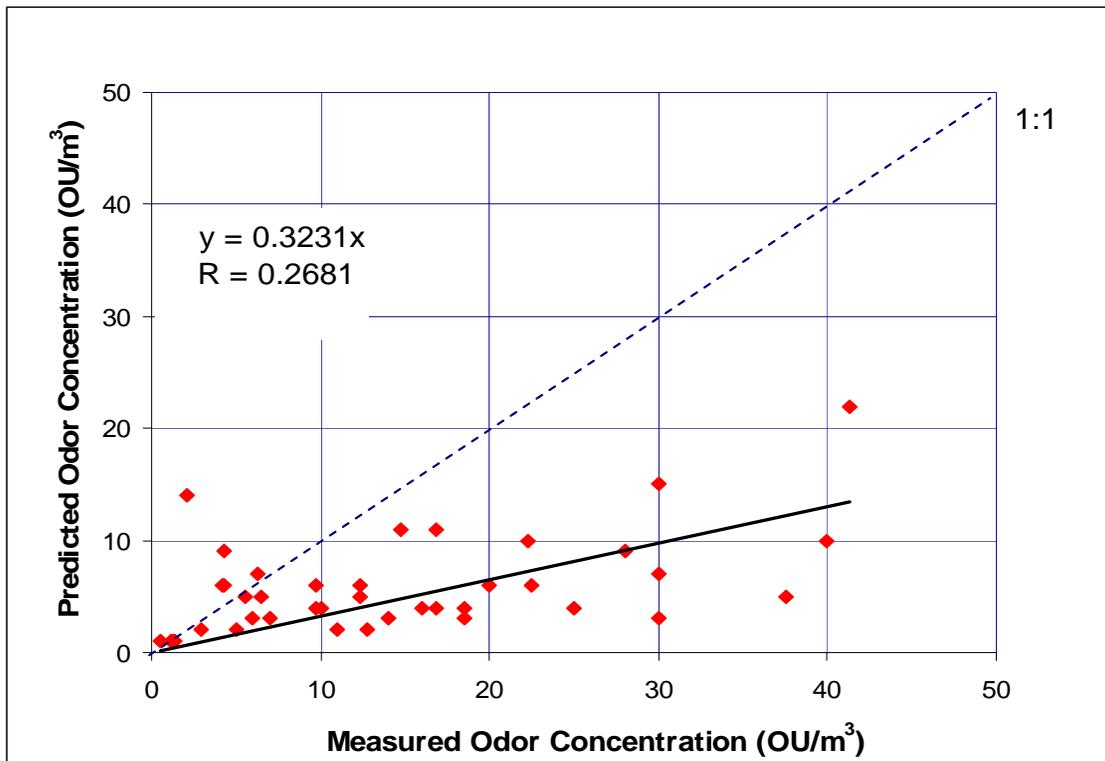
**Figure 3. Predicted and measured odor concentrations for volume source.**
