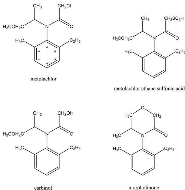
**FIGURE 2. Chemical structures of metolachlor and selected metabolites. Asterisk indicates position of the radiolabel.**
