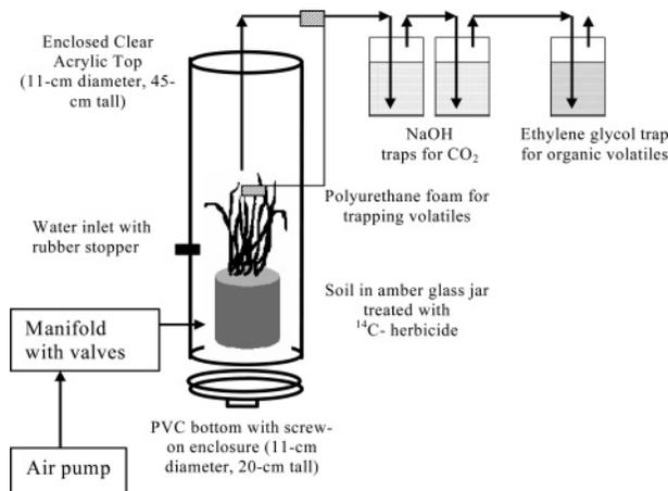
**FIGURE 1. Schematic of enclosed chamber system, with arrows indicating direction of air flow through tubing.**
