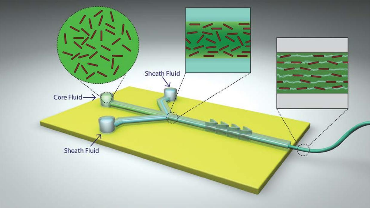
**Figure 1.** Schematic illustration of microfluidic fiber fabrication
