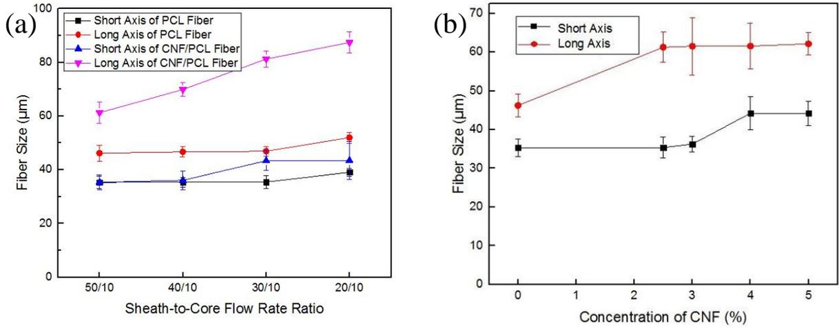
**Figure 4.** Dimensions of fibers with (a) pure PCL and 2.5 wt.% CNF/PCL made with different sheath-to-core flow rate ratios. (b) Fibers with different concentrations of CNF made with sheath-to-core flow rate ratio of 50:10.
