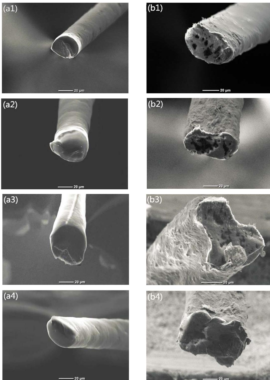
**Figure 3.** Cross-sectional SEM images of (a1-a4) PCL fibers (sheath-to-core flow rate ratio: a<sub>1</sub>-a<sub>4</sub>: 50:10, 40:10, 30:10, 20:10, respectively), (b) 2.5 wt.% CNF/PCL fibers (b<sub>1</sub>-b<sub>4</sub>: 50:10, 40:10, 30:10, 20:10, respectively). (c) 3 wt.% CNF/PCL(50:10).
