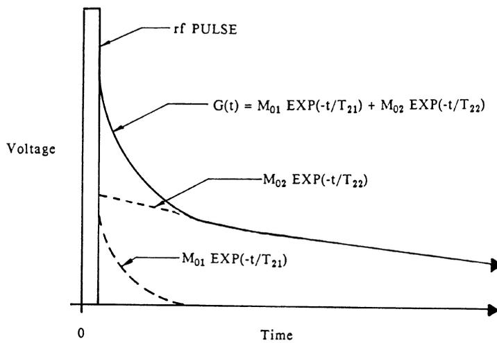
Fig. 3. Shape of two-component NMR free induction decay.
