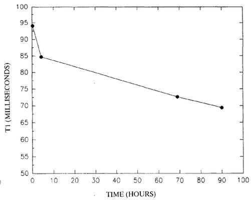
Fig 7.  $T_1$  versus cure time for adhesive liner.
