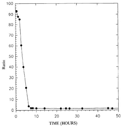
Fig. 6. Ratio of  $M_{01}$  to  $M_{02}$  versus cure time.
