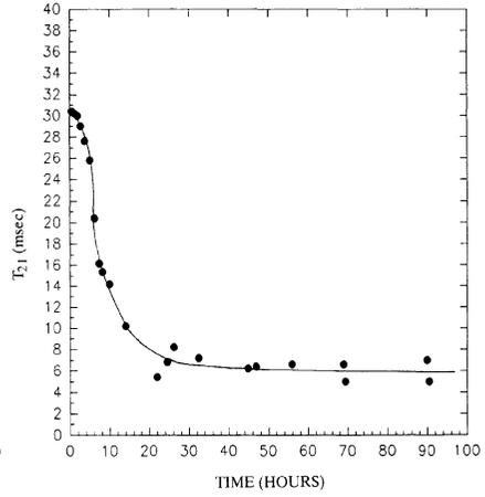
Fig 5.  $T_{21}$  versus cure time.
