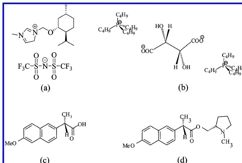
**Figure 1.** Structures of (a) the chiral *N*-methylimidazoliummethyl menthylether bis(trifluoromethylsulfonyl)imide ionic liquid. (b) *L*-Dianionic tartrate ionic liquids with TBP (tetrabutylphosphonium) counter cations. (c) (*S*)-(+)-6-Methoxy-2-naphthylpropionic acid [*S*-naproxen, (*S*)-NPX]. (d) (*S,S*)-*N*-Methyl-2-pyrrolidinemethyl 2(*S*)-(6-methoxy-2-naphthyl) propionate [(*S,S*)-NPX–PYR].
