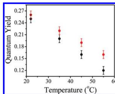
**Figure 3.** Plot of singlet quantum yields against temperature of the (*S,S*)-NPX-PYR dyad in D- (black dots) and L- (red dots) tartrate ionic liquids, obtained from the steady-state emission spectra, taking tryptophan in buffer (pH 7.0) as the standard ( $\Phi_{\text{trp}} = 0.18$ ).<sup>34–36</sup> The error bars are based on the average of three measurements. The fluorescence quantum yields are almost same at 22 °C, but they increasingly differ with temperature.
