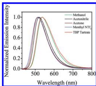
**Figure 7.** Normalized steady-state emission spectra of C153 in different solvents. The fluorescence spectra were obtained by exciting the sample at 420 nm with a 2-nm bandpass. From the peak maxima, the order of polarity of the solvents is: menthyl ILs < acetone < acetonitrile < tartrate ILs  $\approx$  methanol. The  $E_T(30)$  values of the menthyl ionic liquids are 41.1 and 41.3, and those of tartrate ionic liquids are 53.3 and 53.5.
