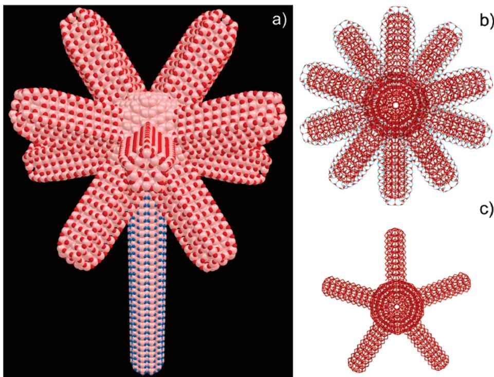
**Figure 2.** (a) SiNF with 10 petals covered by oxidized layers (oxygen atoms are in red and silicon atoms are in pink) and the stalk covered by hydrogen atoms (in blue). The petals and the stalk are attached to the SiIQD1100. (b) SiNF with 10 petals covered by an oxidized layer. The silicon atoms are in burgundy, and oxygen atoms are in green. (c) Silicon nanoflower with 5 petals.
