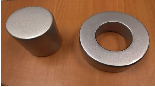
Fig. S1. Image of the BAAM 70 vol.% Nd-Fe-B bonded magnets.
