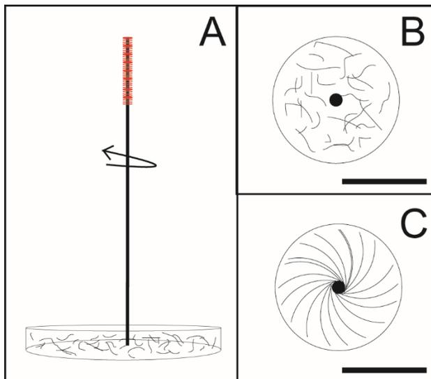
**Figure 1: Schematic of aligned collagen gels.** (A) An acupuncture needle is inserted into a collagen gel and rotated. A top view of the needle in the gel (B) before rotation and (C) after rotation. The scale bars are 1 cm.
