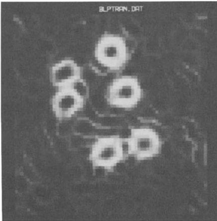
Fig. 6. Low-pass transformation applied to the image in fig. 2(a).
