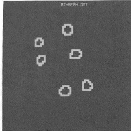
Fig. 7. Thresholding plus Roberts filter applied to the image in fig. 2(a). The result is the binary image of the defect contours.
