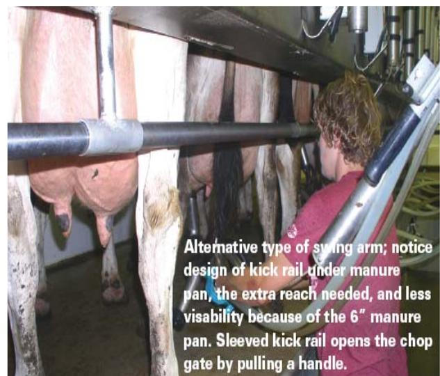
Alternative type of swing arm; notice design of kick rail under manure pan, the extra reach needed, and less visibility because of the 6" manure pan. Sleeved kick rail opens the chop gate by pulling a handle.
