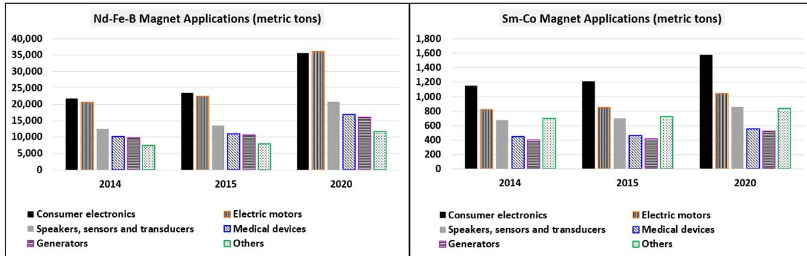
Fig. 1: 2014, 2015 and 2020 (forecasted) applications of Nd-Fe-B and Sm-Co PMs (*plotted with data from [5]*).
