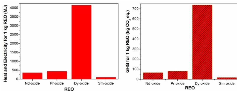
Fig. 3: Energy and greenhouse gas emission associated with the production of 1 kg of primary REOs:  $\text{Nd}_2\text{O}_3$ ,  $\text{Pr}_6\text{O}_{11}$ ,  $\text{Sm}_2\text{O}_3$  and  $\text{Dy}_2\text{O}_3$ , for magnet production. (plotted with data from [44]).
