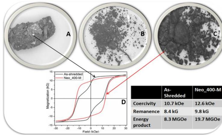
Fig. 6: Demonstrating the possibility to reuse magnets from shredded HDDs showing: (A) Magnet manually concentrated from as-shredded HDD; (B) Material derived from demagnetizing the magnet concentrate; (C) Magnet separated from other components of the mix; (D) Magnetic hysteresis loops of the magnet concentrate (black plot) and the separated magnet (red plot). Inset: Magnetic properties derived from the hysteresis loops.
