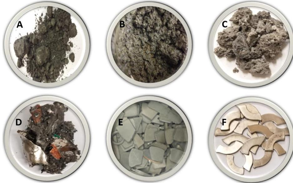
Fig. 5: Forms of feedstock materials for PMs recycling: (A). Dry grinding swarfs (B). Wet grinding swarfs (C). Slags (D). Shredded electronic waster from HDD (E). Scrap magnets and (F) HDD magnets.
