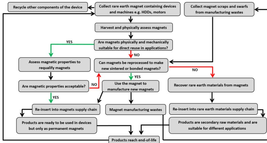
Fig. 4: Decision diagram illustrating circular economy for recycling REEs from permanent magnets materials contained in devices and magnet manufacturing plants.
