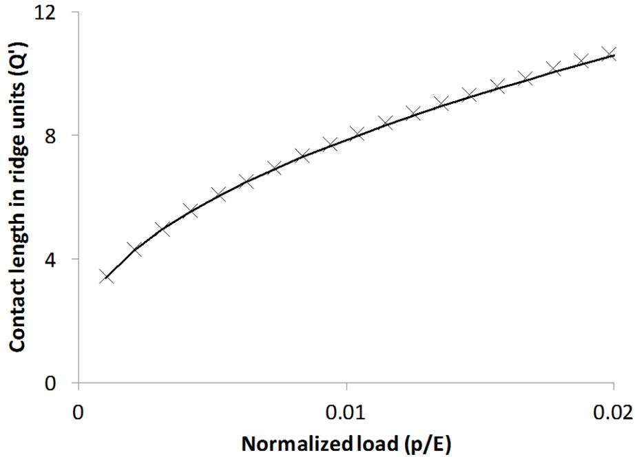
Figure 3. The points represent the computational model's contact length between a cylinder and two rigid planes expressed as total ridge units in contact ( $Q'$ ) using (2) at values  $a/R = 0.022$  and  $b/R = 0.03$ . The simulated results are predicted with high accuracy ( $R^2 \approx 1$ ) by the classic Hertzian contact (solid line).
