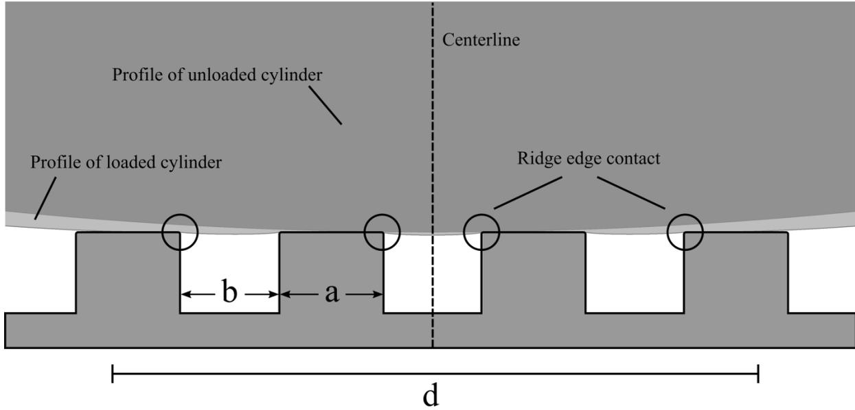
**Figure 1. Illustration of the ridge geometry used in this study. ‘d’ is the overall contact distance, ‘a’ is the ridge width, and ‘b’ is the groove width. In this figure, the unloaded cylinder is in initial contact with 2 proximal ridges, ( $Q = 2$ ). Under load,  $Q$  increases to 4 ridge edges in contact with the cylinder.**
