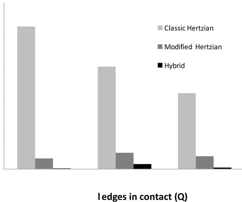
**Figure 6. Percent error of required load for number of ridge edges in contact for large groove width ( $b/R=0.03$ ) and small ridge width ( $a/R = 0.012$ ). At these higher ratios of  $b/R$  to  $a/R$ , the Classic Hertzian prediction become extremely inaccurate. The Modified model is also challenged, but the Hybrid model remains highly accurate.**
