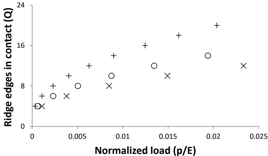
**Figure 4.** Number of proximal ridge edges in contact as a function of load, with  $b/R = 0.01$  and  $a/R$  ranging from 0.032 (X), to 0.022 (O), and 0.012 (+). This plot is representative of the behavior of the other test combinations.
