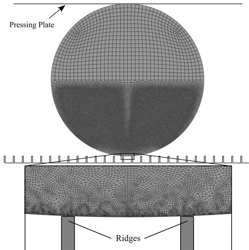
**Figure 2. Illustration of the configuration used in the finite element model, with a large  $b/R$  of 0.09, and small  $a/R$  of 0.011. The mesh is highly refined at the area of contact. The lower part of the figure shows greater detail of the ridges.**
