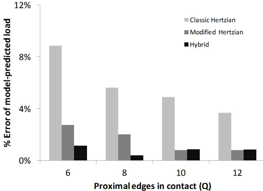
**Figure 5. Percent error of model-predicted load for a specific number of proximal ridge edges in contact, for small groove width ( $b/R=0.01$ ) and large ridge width ( $a/R=0.032$ ). While the Classic and Modified Hertzian models performed well, they were outperformed by the Hybrid Model.**
