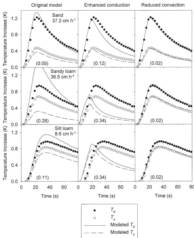
**Fig. 6.** Measured temperature increases at the highest water flow rate for sand, sandy loam, and silt loam soil and modeled temperature increases using the original model ( $a = b = 1$ ), an enhanced conduction model ( $a = 1/S$ ), and a reduced convection model ( $b = S$ ). Root mean square error (K) is shown in parentheses at the bottom of each pane.
