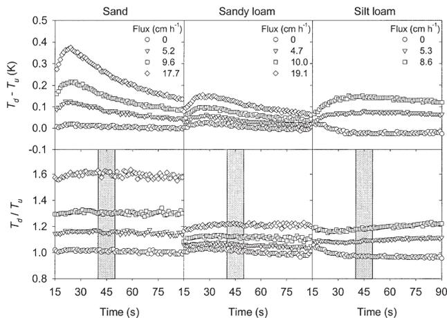
**Fig. 1.** Samples of measured temperature increase differences (top panel) and temperature increase ratios (bottom panel) in sand, sandy loam, and silt loam soil for water fluxes from 0 to 20 cm h<sup>-1</sup>. The shaded regions in the bottom panel indicate the time window over which the temperature increase ratio was averaged.
