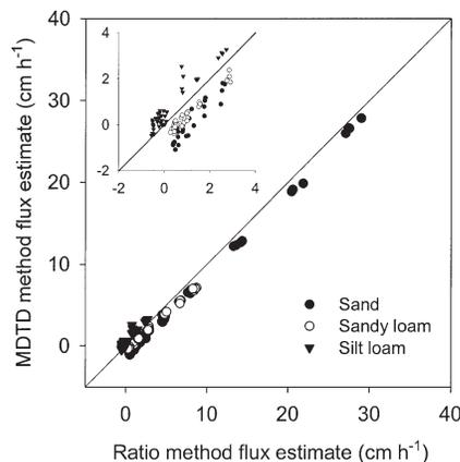
**Fig. 4.** Comparison of water flux estimated by the maximum dimensionless temperature increase difference (MDTD) method with water flux estimated by the ratio method. The inset expands the scale at the low end.
