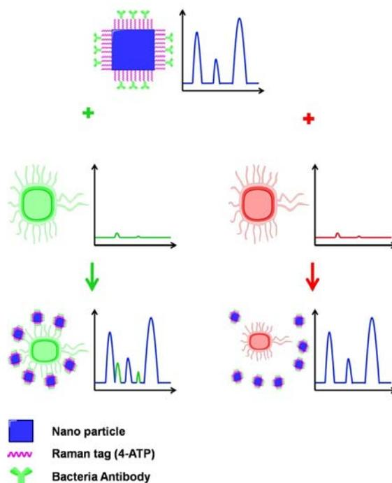
Fig. 1 Scheme of dual recognition bacterial detection SERS nano probe
