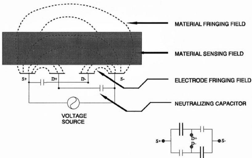
Figure 1. One-sided absolute capacitive bridge probe.
