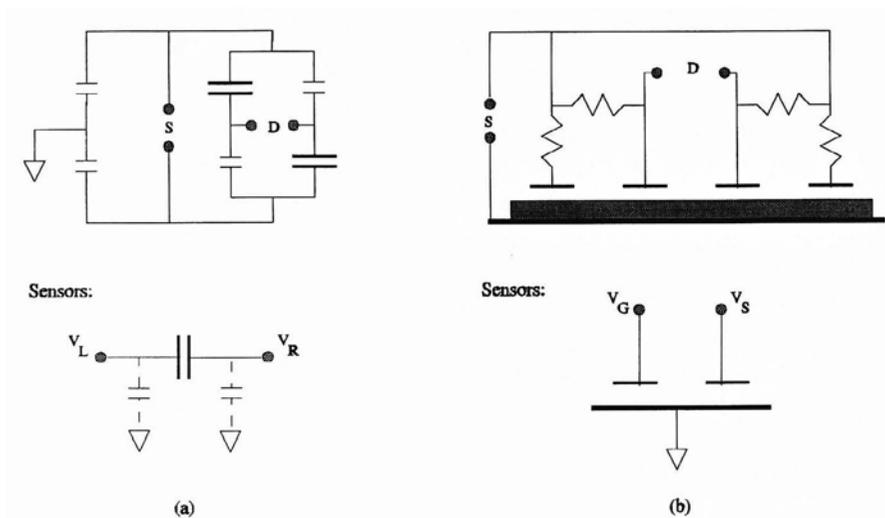
Figure 3. Equivalent circuit modeling: (a) one-sided absolute probe and (b) feed-through differential probe.
