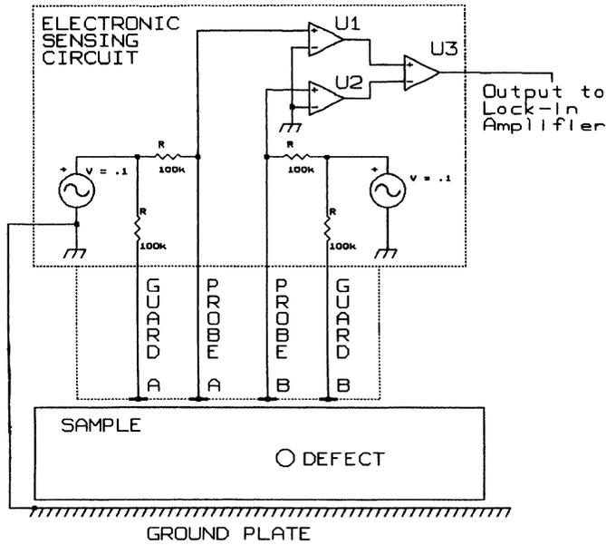
Figure 2. Feed-through differential capacitive probe.
