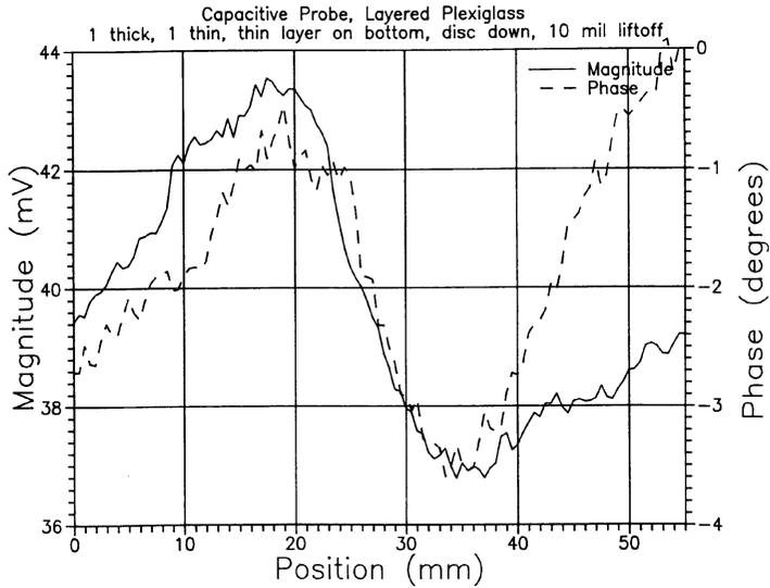
Figure 5. Surface scan of a horizontal penny-shaped void (6.35 mm radius by 1.02 mm thickness in acrylic plastic (PMMA) at 0.00 mm depth and 0.25 mm liftoff with the feed-through differential probe, Figure 3).
