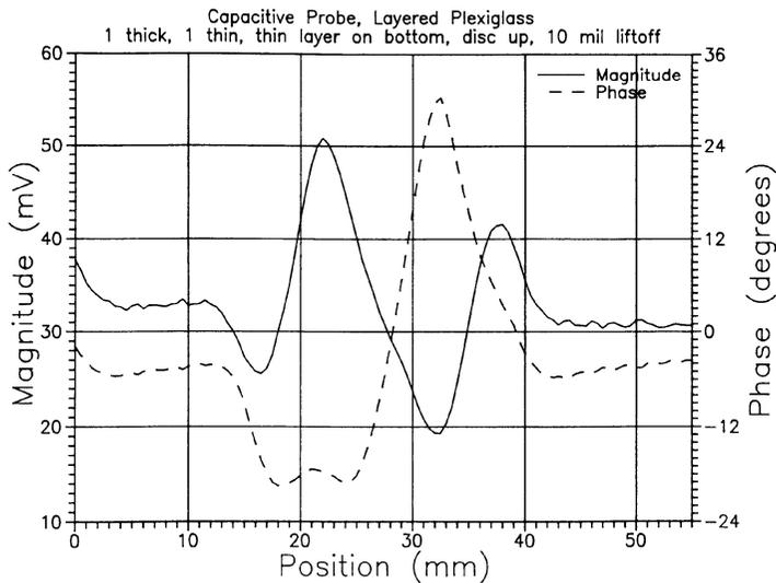
Figure 6. Surface scan of the same defect at 12.7 mm depth and 0.25 mm liftoff with the same probe as used in Figure 5.
