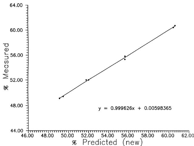
Figure 4. Density calibration curve for ceramic green-state compaction measurements with the one-sided absolute probe (Figure 1).
