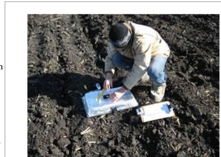
Static flux chamber (pictured) method was developed to measure greenhouse gas emissions from land-applied swine manure from a corn-on-corn system in central Iowa in the Fall of 2012. Gas samples were collected in vials and transported to
