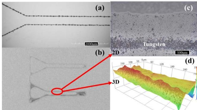
**Figure 7.** (a) Optical image. (b) x-ray radiography image of printed tungsten lines with 20 layers (top) and 50 layers (bottom). (c) and (d) are magnified 2D and 3D images of the 50 layers tungsten line, respectively.
