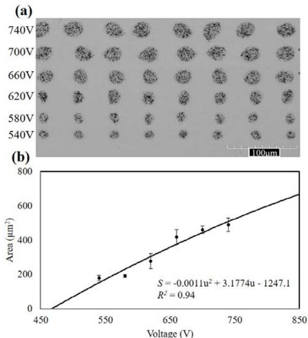
**Figure 4.** Printed tungsten dots with e-jet printing in different voltages. (a) optical microscope image, (b) dots area as a function of printing voltage.
