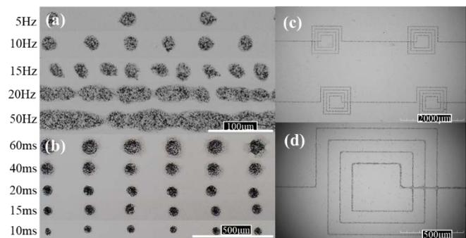
**Figure 5.** Optical microscope images of tungsten dots under different (a) frequencies and (b) pulse widths of high voltage; Optical microscope images of tungsten shaped lines with (c) low and (d) large magnification.
