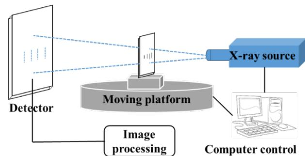
**Figure 2.** Schematic of the lab-built x-ray imaging system.
