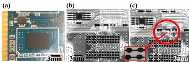
**Figure 9.** (a) Optical image of circuit board. (b) x-ray radiography image of the circuit board. (c) Printed capacitor and cover patterns on the circuit board under x-ray imaging
