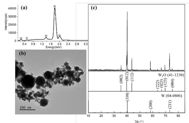
**Figure 3.** (a) Energy dispersive spectroscopy (EDS) and (b) transmission electron microscopy (TEM) images of tungsten nanoparticles. (c) X-ray diffraction (XRD) results of printed tungsten dots.
