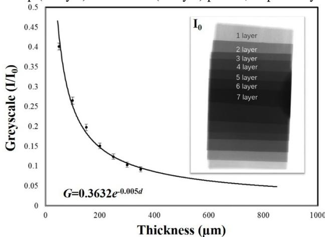
**Figure 8.** Grayscale of bulk tungsten sheet as a function of its thickness. The inset is an x-ray radiography image of tungsten sheets with different layers.
