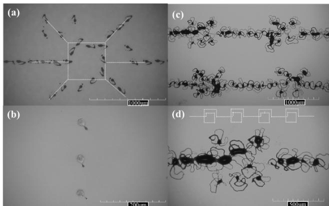
**Figure 6.** Optical microscope images of tungsten patterns at different conditions: (a) DC voltage and the dashed lines were the designed pattern; (b) large pulse width with AC voltage; (c) and (d) are non-fresh ink with normal and high voltage at the designed patterns as dashed lines in inset. The dashed lines denote designed printing path.
