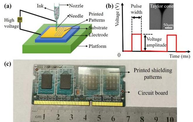
**Figure 1.** (a) Schematic of e-jet printing. A high voltage is applied between the needle and plate electrode. (b) Voltage modality and a machine vision of e-jet printing process. (c) A typical circuit board partially covered by printed patterns for the radiation shielding concepts.
