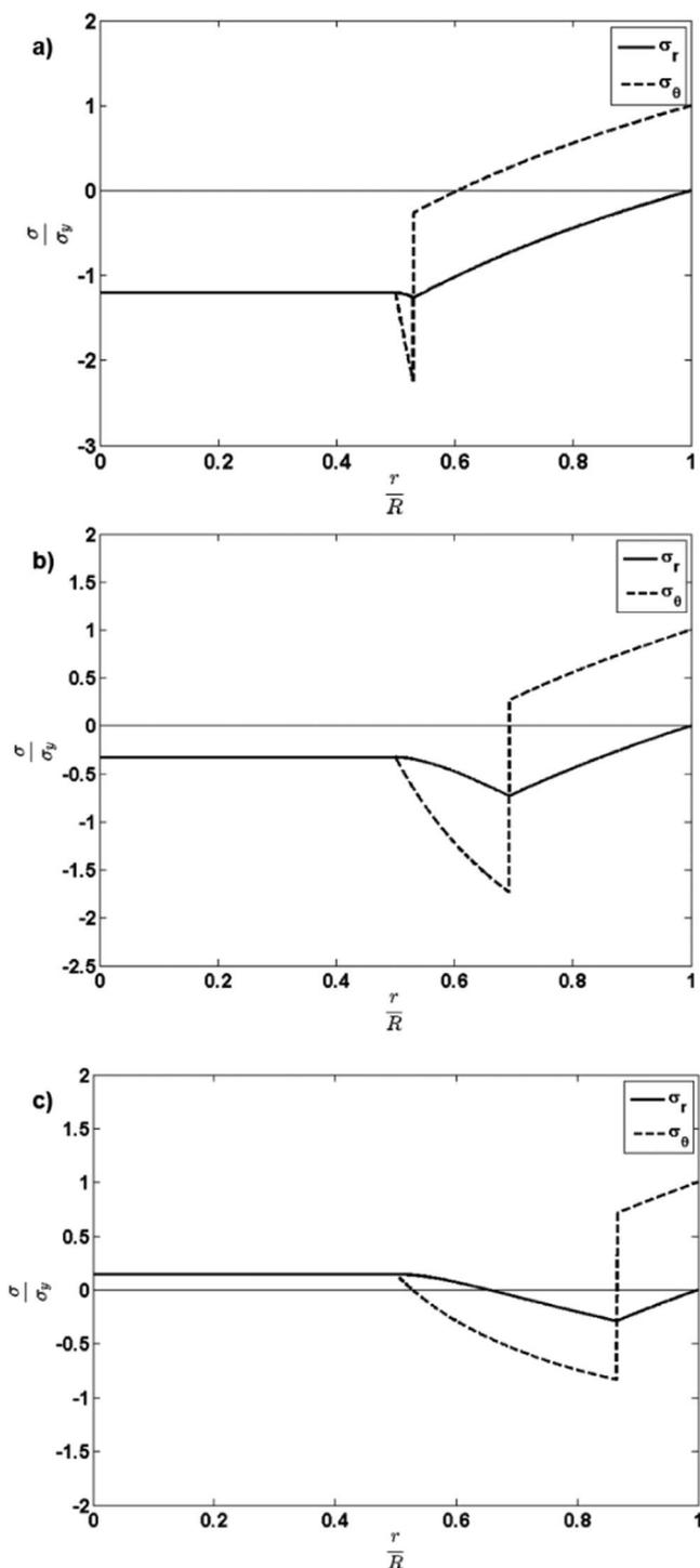
**Figure 4.** Normalized stress (radial and hoop) vs normalized radius (200 nm) for different elastic moduli a) 80 GPa b) 24.5 GPa c) 12 GPa.
