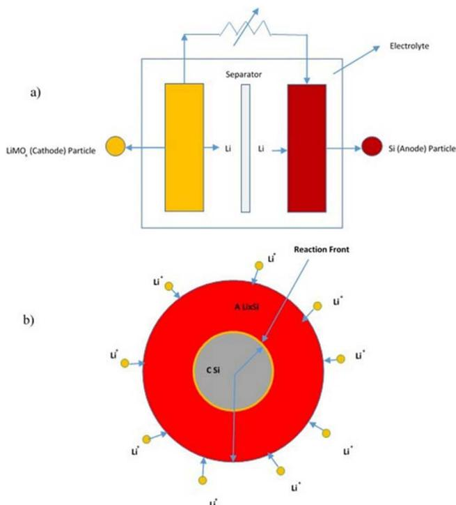
**Figure 1.** a) Schematic of lithium-silicon battery. b) Diffusion-Reaction Mechanism of lithium during charging in silicon nanoparticle.
