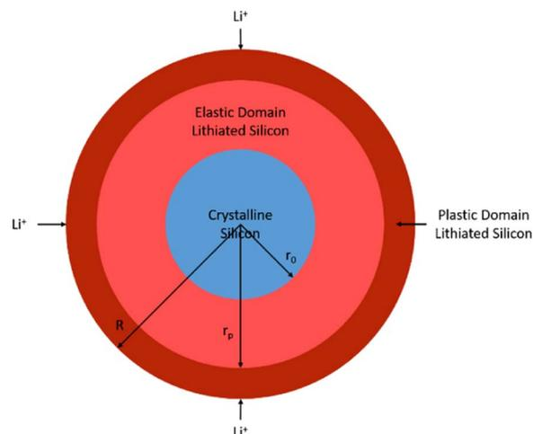
**Figure 2.** Schematic of stress domain in partially lithiated silicon particle battery.
