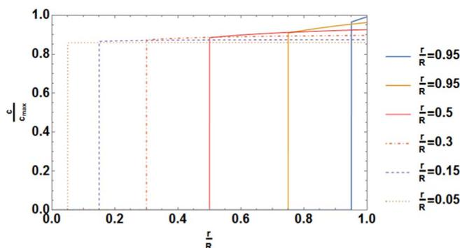
**Figure 3.** Normalized concentration vs normalized radius variation at different stages of penetration of reaction front into silicon particle.
