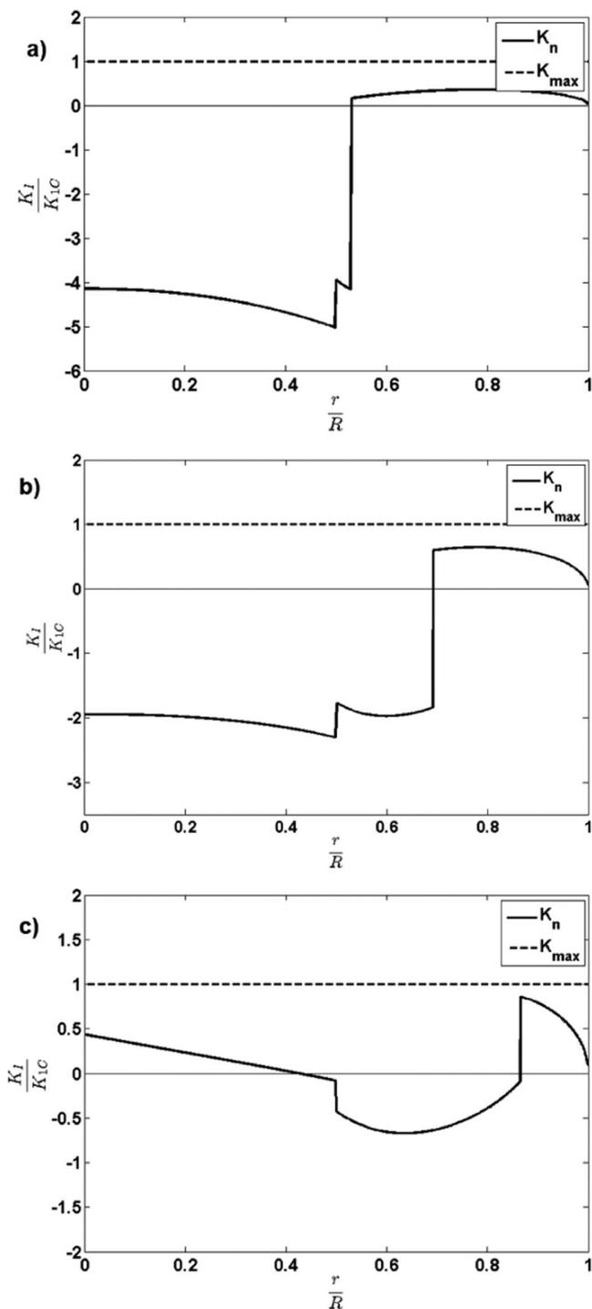
**Figure 5.** Normalized stress intensity factor vs normalized radius (200 nm) for different elastic moduli a) 80 GPa b) 24.5 GPa c) 12 GPa.
