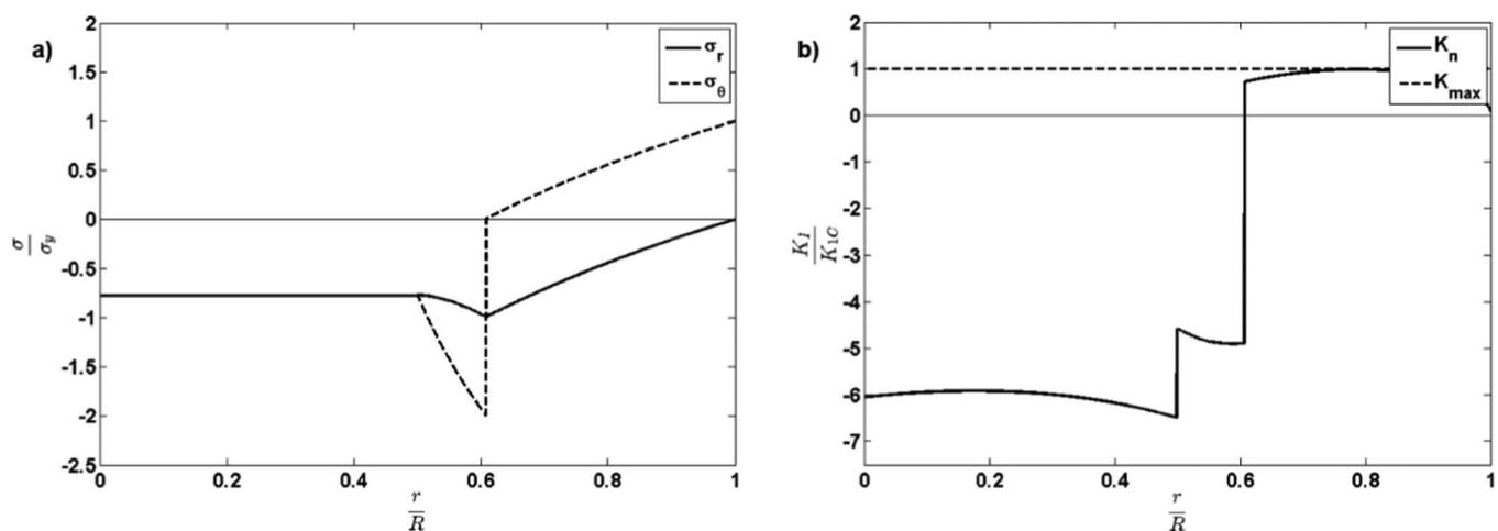
**Figure 7.** a) Normalized stress (radial and hoop) vs normalized radius (450 nm) for 24 GPa b) Normalized stress intensity factor vs normalized radius (450 nm) for 24 GPa.
