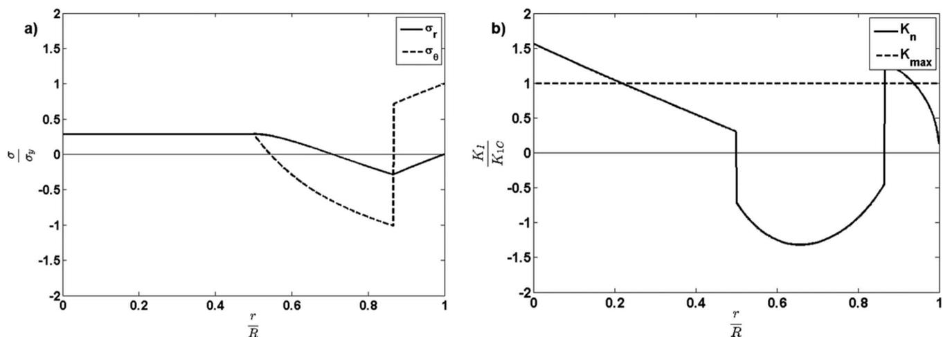
**Figure 6.** a) Normalized stress (radial and hoop) vs normalized radius (450 nm) for 12 GPa b) Normalized stress intensity factor vs normalized radius (450 nm) for 12 GPa.
