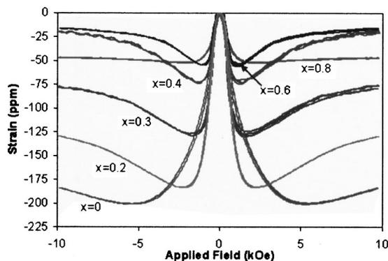
FIG. 3. Magnetostriction curves for  $\text{CoFe}_{2-x}\text{Mn}_x\text{O}_4$  samples.
