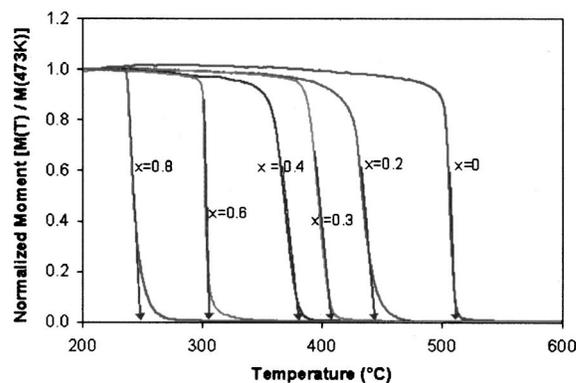
FIG. 1. Normalized magnetic moment vs temperature upon cooling for pure cobalt ferrite and manganese-substituted cobalt ferrite samples CoFe<sub>2-x</sub>Mn<sub>x</sub>O<sub>4</sub> with various manganese contents ( $x=0$  to 0.8).
