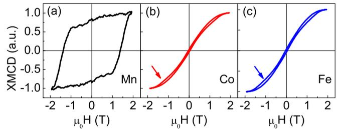
FIG. 3. X-ray magnetic circular dichroism (XMCD): Out-of-plane element-sensitive XMCD hysteresis loops for MnBi (20 nm)/Co<sub>0.7</sub>Fe<sub>0.3</sub> (5 nm) Mn (a), Co (b), and Fe (c).
