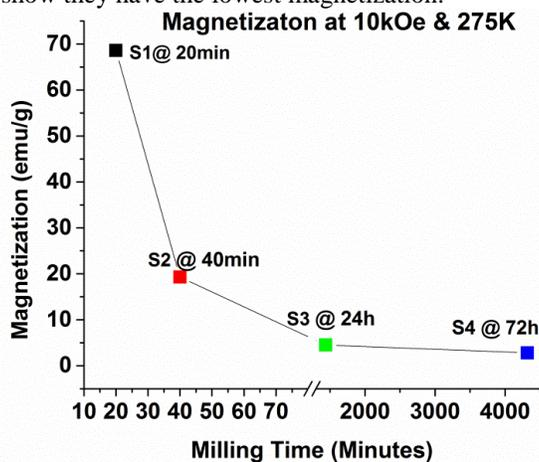
**FIG. 8** Magnetization vs. milling time at 275 K and 10kOe for all the samples; S1 through S4 show that magnetization decreases significantly with increase in milling time which can also be observed from Fig 4 and Fig. 7.
