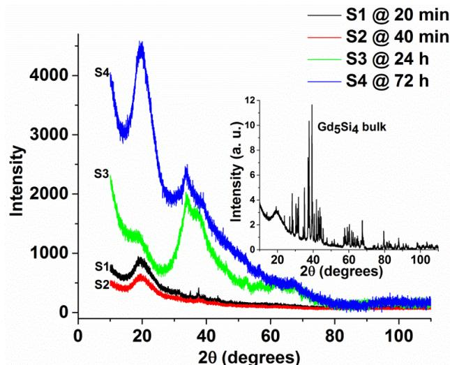
**FIG. 2** XRD patterns for S1, S2, S3 and S4 samples under different milling conditions. Inset shows XRD peak patterns for bulk  $Gd_5Si_4$ .
