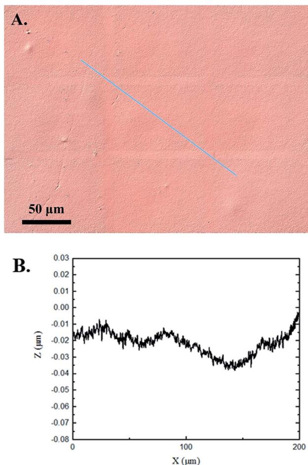
**Fig. 2** 3D confocal microscopy analysis of a control PDMS sample. (A) The surface is visibly flat with some minor surface impurities. (B) Graphical height displacement across an arbitrary line on the surface.
