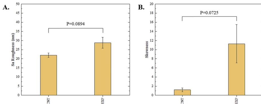
Fig. 4 Summary of (A) average  $S_a$  and (B) average  $S_{sk}$  roughness parameters of control and experimental samples via 3D confocal microscopy techniques. Error bars represent the standard error of the mean.  $N = 5$ .
