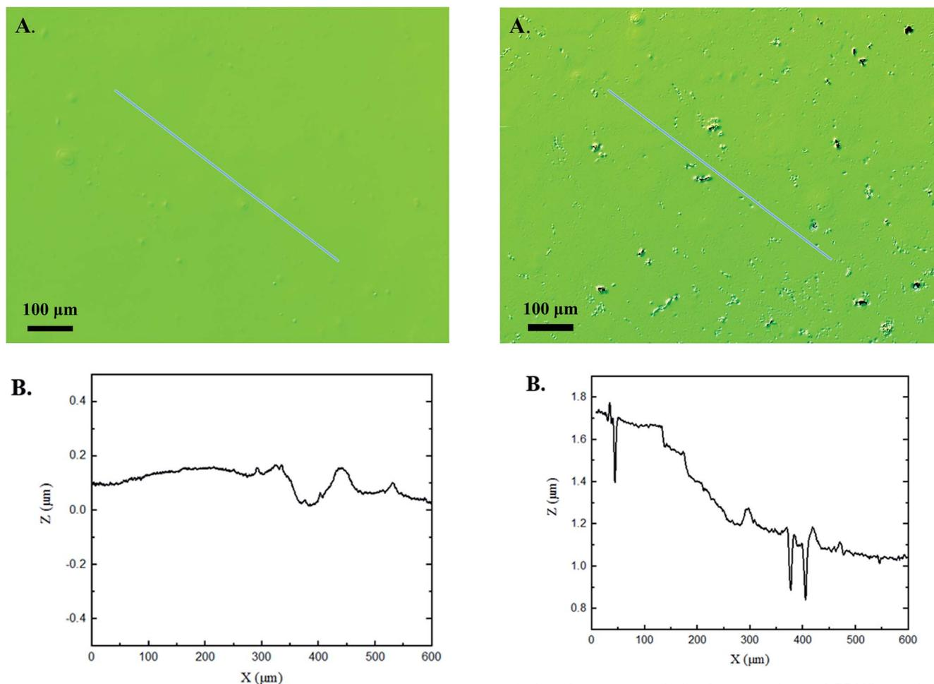
Fig. 5 Interferometry analysis of a control PDMS sample. (A) The surface is visibly flat with some minor surface impurities. (B) Graphical height displacement across an arbitrary line on the surface. Any abrupt spikes in the z direction appear to be above the surface.
